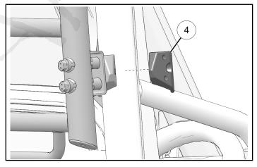
Loosely attach right ROPS clamp 4 using screw
