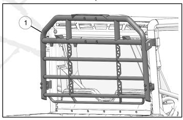
2. Put steel spacer <sup>(9)</sup> between headache rack mount and mounting bracket on ROPS.
