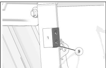
3. Install hinge plate ② on inside face of hinge bracket. Hold hinge plate in place.
