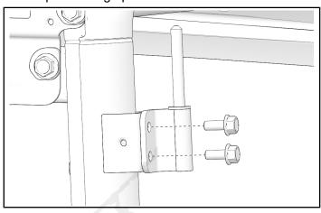
4. Put headache rack 1 in position on vehicle.
