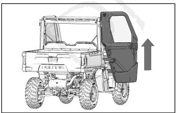
3. Remove and discard two screws. Remove and keep door hinge pin.
