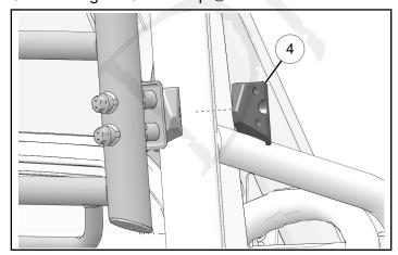
9. Loosely attach right ROPS clamp @using screw (5)
