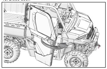
14. Connect rubber limiter strap from door. Connect any electrical connectors between door and vehicle.
