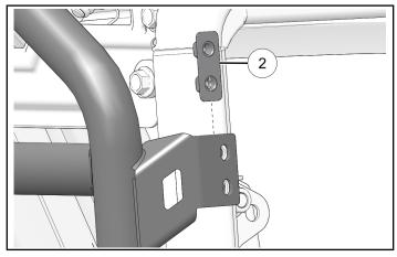
6. Install door hinge pin between headache rack ① and mounting plate on ROPS.
