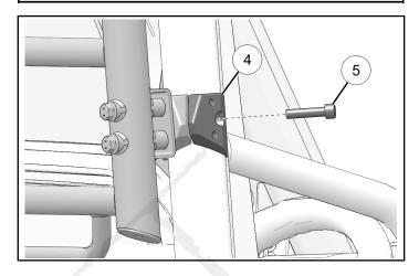
10. Torque two ROPS clamp screws ⑤ to specification.
