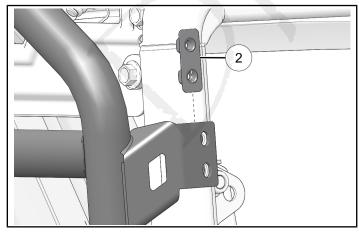
4. Loosely attach headache rack using two washers ③ and two screws ⑥. Install screws into hinge plate ② (not shown).
