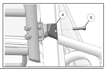
7. Torque two ROPS clamp screws ⑤ to specification.
