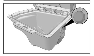
3. Put socket ② through hole. Use socket ② as a template to mark two screw holes. Remove socket.
