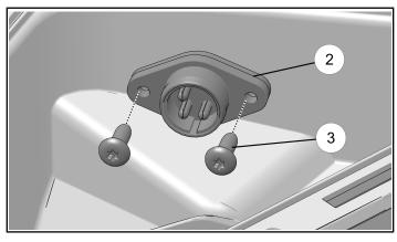
2. Connect socket ② to winch harness. Turn storage compartment to reach wire harness.
