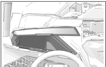
2. Install six storage compartment fasteners. Torque fasteners until fully seated.
