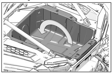
2. Loosely install stepped washers and attach to cargo box with two screws. Torque screws to specifications.
