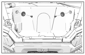
3. Insert two screws and attach cargo box to vehicle. Torque screws to specifications.
