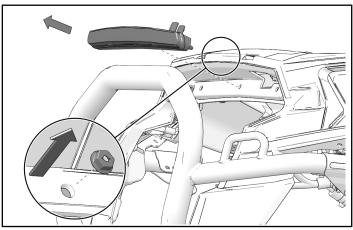
2. Attach front accent light assembly ① with three hex nuts ②. Torque nuts to required specification.
