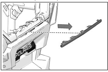
5. Insert center accent light ③ to vehicle with four hex nuts. Torque nuts to required specification. ②.
