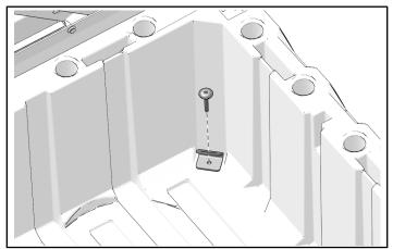
2. Drill a 5/16 in (8 mm) hole in each corner at the dimple.
