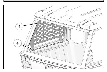
Install upper mounting hardware. Use screw (5) and nut (6) in hole closest to front of vehicle. Use screw (5), nut (6), and spacer (3) in hole closest to rear of vehicle. Position spacer between MOLLE panel and enclosure, as shown. Torque screws to specification.
