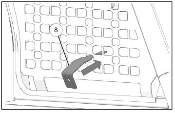
6. Push bottom of leg (8) toward rail, and lower leg until it rests on rail.
