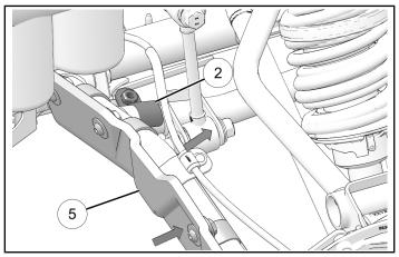
10. Install screw (9) and washer (12) for side clamp from underside of guard (5).
