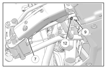
5. Install bracket ④ on front of control arm. End of bracket will pass through wire mount on control arm.
