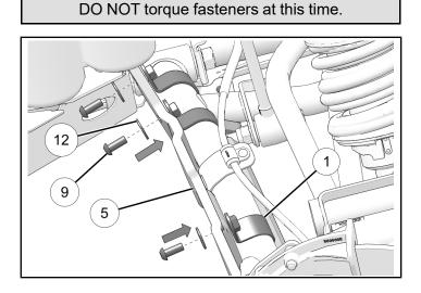
DO NOT torque fasteners at this time.
