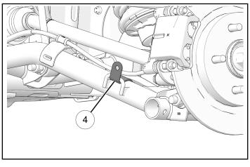
6. Install arm guard 5 on front of control arm. Install two screws 9 and two washers 12 through guard 5 and bracket 4.
