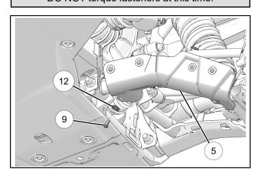
DO NOT torque fasteners at this time.
