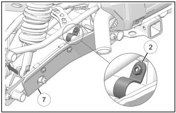
4. Install screw (9) and washer (12) for side clamp from underside of guard (7).
