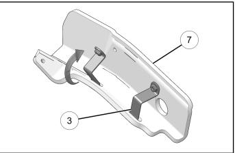
Install guard ⑦ onto rear side of control arm. Wrap clamps around tube. Install two screws ⑨ and two washers ⑫.
