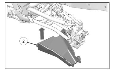
2. Loosely install three screws ③, washers ④, and clamps ⑤ on front side of guard.
