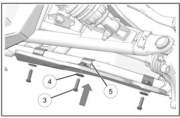
3. Loosely install three screws ③, washers ④, and clamps ⑤ on rear side of guard.
