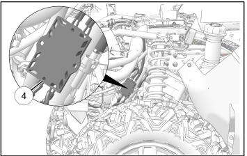
2. Install wireless receiver ③ on upper body bracket. Install cables along frame tube as shown. Attach wireless receiver with cable ties.
