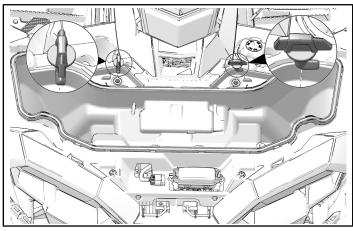
4. Install storage bin cover and secure with straps.
