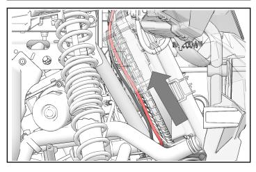
4. Install four screws ④ and torque to specification.
