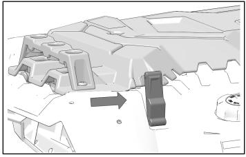
2. Remove two fasteners from front storage bin. Remove front storage bin.
