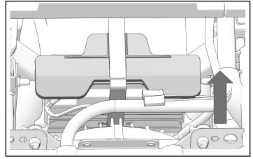
4. Remove bolt from black negative battery cable and disconnect negative battery cable. Remove bolt from red positive battery cable and disconnect positive battery cable.
