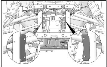
2. Put winch in position on vehicle, lining up four mounting points. Make sure not to pinch any wires.
