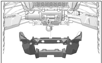
2. Install four retained bolts and torque to specification.
