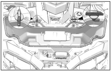
3. Fold up ends of battery cover to access battery bolts.
