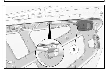
9. Align door panel mounting holes with frame and install the nine retained fasteners. Torque fasteners to specification.
