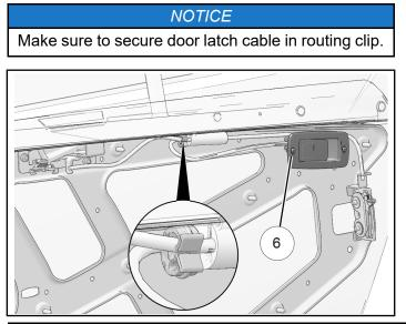
9. Align door panel mounting holes with frame and install the nine retained fasteners. Torque fasteners to specification.
