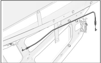
8. Place door near door frame and install door handle cable onto inner door actuator and handle.
