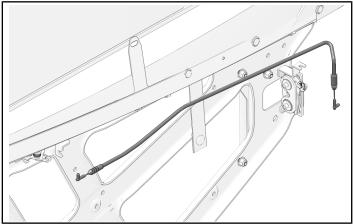
8. Place door near door frame and install door handle6 cable onto inner door actuator and handle.
