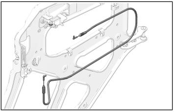
8. Place door near door frame and install door handle cable (5) onto inner door actuator and handle.
