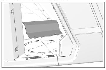
2. Install tunnel cover with four retained push-pin rivets.
