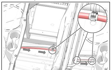
8. Route the positive battery cable towards the battery and install to the chassis with attached push darts.
