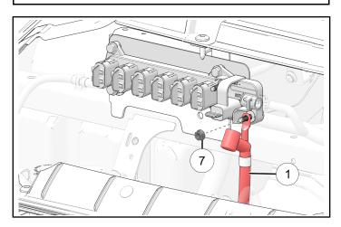
5. Install three attached push-darts to the vehicle chassis.
