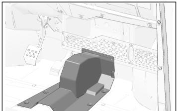
2. Install tunnel cover with six retained push-pin rivets
