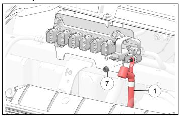
2. Put electrical mounting panel ③ in the vehicle and put the positive battery cable through the opening in the panel.
