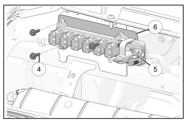
2. Remove and discard the cap from the chassis harness connector.
