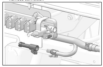
3. Install the chassis harness connector to the Polaris Pulse® bar.
