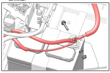
2. Install positive battery cable to battery terminal with retained hardware. Counter-hold nut and torque one bolt to specification.
