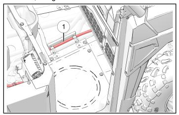
2. Route one end of the cable towards the front of the vehicle and install one push dart into the chassis.
