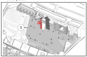
3. Install positive battery cable ① to the Polaris Pulse® bar with one nut ⑦. Torque nut to specification.
