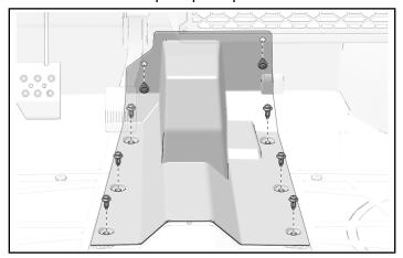
2. Remove tunnel cover from vehicle.
