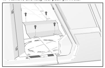
2. Remove rear tunnel cover from vehicle.
