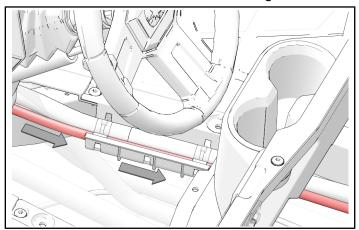
7. Crew Models Only: Route positive battery cable alongside the chassis electrical harness in the harness trough. Attach with clips where available.
