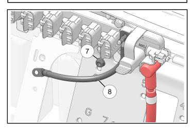
2. Install the ground cable (8) to the vehicle chassis with one screw (4). Torque one screws to specification.
