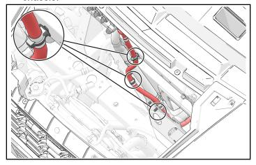
6. Route positive battery cable alongside the chassis electrical harness in the harness trough.
