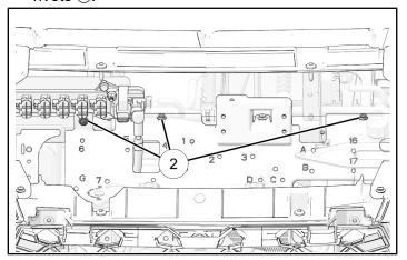
5. Install bottom of mounting panel with two push-pin rivets ②.
