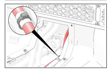
3. Pull the positive battery cable from the tunnel.
