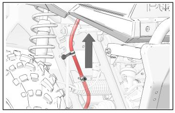
4. Loosely install positive battery cable 1 to the Polaris Pulse® bar with one nut 7.
