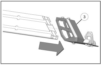
6. Install Rhino Rack® Accessory into desired slot in rail ②.
