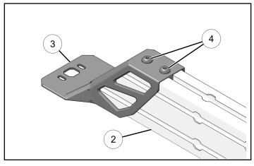
3. Install Lock & Ride MAX® latching assembly ① as shown.
