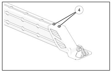
4. Loosen screw ④ on bottom of rail mount. Do not remove screw from T-nut in rail.
