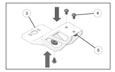
2. Loosely assemble mount ③ to crossbar rail ②. Do not tighten screws ④.
