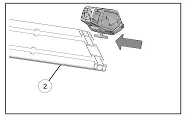
7. Move Rhino Rack® Accessory to desired location. Tighten screw on accessory to hold accessory in desired location.
