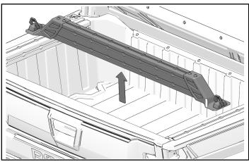
3. Loosen two screws ④ on top of rail mount. Do not remove screws from T-nuts in rail.
