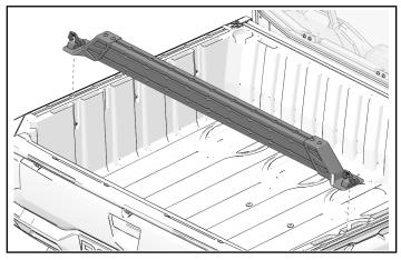
6. If needed, adjust mounts ③ to match the distance from rail to rail. When the mounts are positioned properly, lock latching assembly ① in place by closing the levers.
