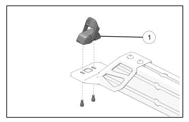
4. Torque latching assembly screws to specification.
