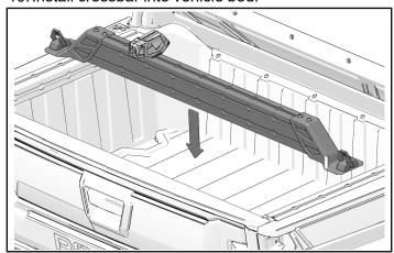
11. Push down latches to close Lock & Ride MAX® latching assemblies.
