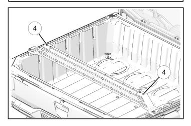
Re-torque latching assembly screws to specification after initial 100-miles of use.
