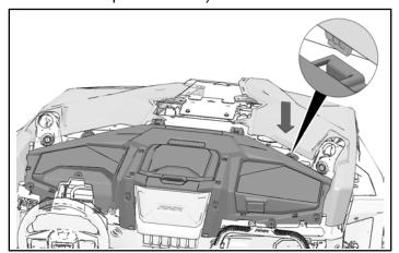
3. Make sure both rubber boots are properly seated around hood panels. Only upper lip should be visible, as shown with inset.
