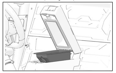
4. Disconnect 12 volt outlet from within center console cavity.
