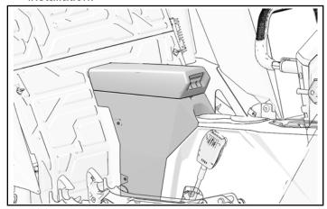
2. Install console storage compartment with two retained center console fasteners from passenger side.
