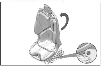
2. Lower seat onto rear receiver tubes.
