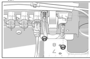
5. Install negative (black) and positive (red) onto Polaris Pulse® bar terminals with retained nuts. Torque nuts to specification.
