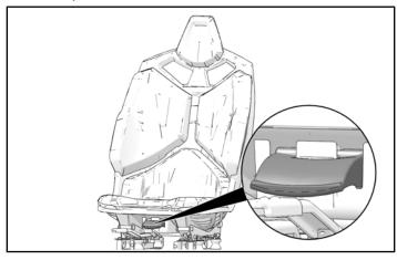
2. Tilt seat assembly forward and pull back slightly to disengage from receiver tube and remove seat from vehicle.
