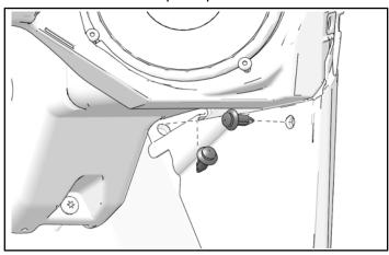
6. Install one screw attaching center console to front dashboard. Torque one screw to specification.
