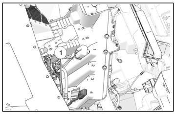
2. Install fuse relay into accessory mounting tray.
