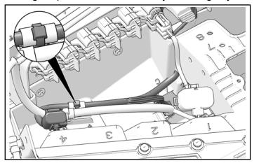
4. Remove and keep two nuts from Polaris Pulse® bar.
