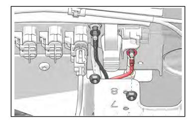
6. Route remaining harness through opening in accessory mounting tray and install connector to main audio harness.
