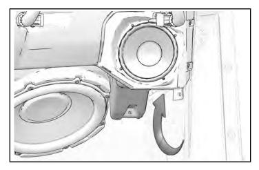
2. Install right-hand speaker with two retained screws. Torque screws to specification.
