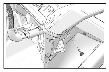
8. Install speaker grille to dashboard with two retained screws.
