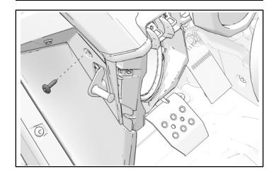
7. Install speaker grille to dashboard with two retained screws.
