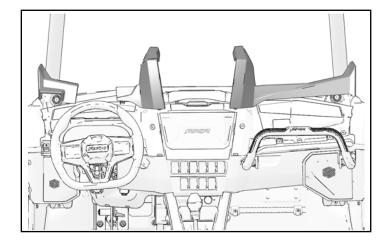
2. Open glove box lid. Remove and keep four dashboard fasteners around glove box opening.
