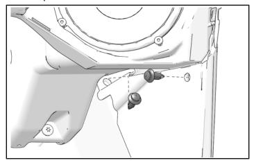
6. Remove and keep four screws attaching front dashboard to speaker.
