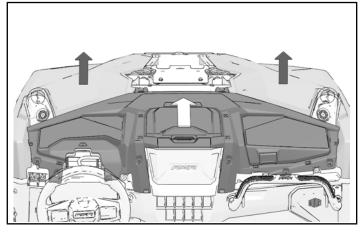
2. Make sure tabs on panels are aligned in slots on dashboard top. (Passenger-side panel shown; driver-side panel similar.)
