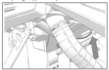
5. Put left-hand speaker connector through an opening in upper fender panel.
