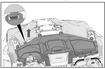
8. Carefully lift edge of right front hood panel to release tab from dashboard top as shown.
