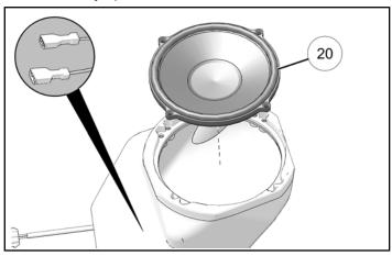
4. Install speaker @ to speaker housing with retained screws. Torque screws to specification.
