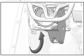
2. Install speaker with two retained screws. Torque screws to specification.
