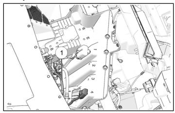
2. Install fuse relay into accessory mounting tray.
