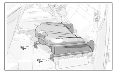
2. Position backrest assembly into seat base and lean back until headrest engages with receiver tube.
