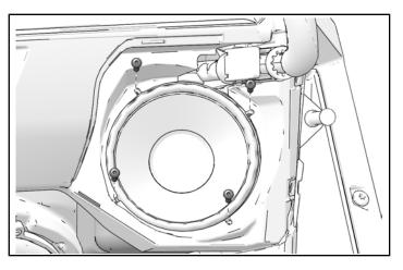
5. Install two retained push-pin rivets.
