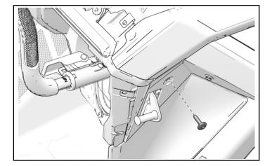
8. Install speaker grille to dashboard with two retained screws.
