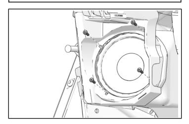
5. Install two retained push-pin rivets.
