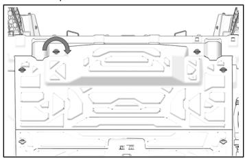
2. Turn each knob 1/4 to disengage and remove bottom close-off panel.
