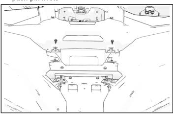
6. Tilt steering wheel down. Install four retained screws through dashboard top and torque to specification.
