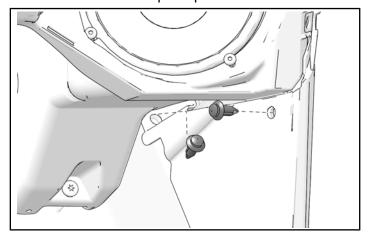
6. Install one screw attaching center console to front dashboard. Torque one screw to specification.
