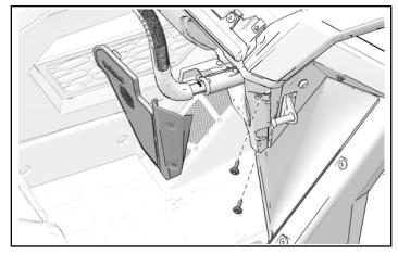
2. Remove and keep one screw attaching fender flare to front dashboard.
