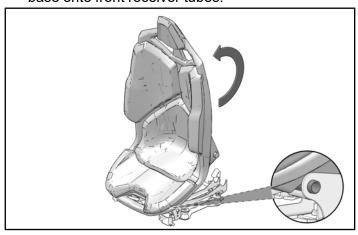
2. Lower seat onto rear receiver tubes.
