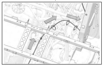
3. Install harness above heat shield with push-darts and cable ties at taped locations.
