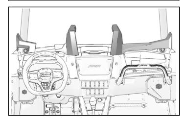
2. Open glove box lid. Remove and keep four dashboard fasteners around glove box opening.
