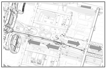
2. Route harness towards left-rear of vehicle and install with cable ties at taped locations
