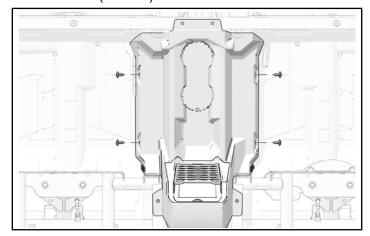
3. Remove and keep four push-pin rivets.
