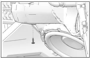
7. Install one screw attaching fender flare to front dashboard. Torque one screw to specification.
