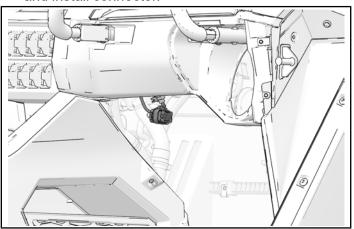
3. Tilt subwoofer, with backside upwards behind front dashboard, into installed position..
