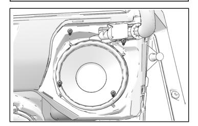
5. Install two retained push-pin rivets.
