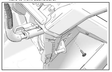
3. Remove and keep one screw attaching center console to front dashboard.
