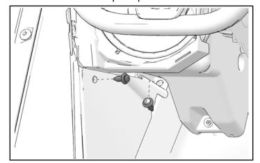
6. Install one screw attaching fender flare to front dashboard. Torque one screw to specification.
