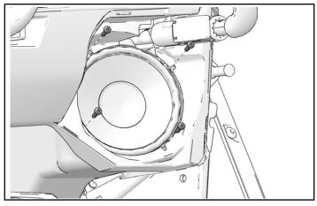
7. Remove and keep two screws attaching speaker to firewall.
