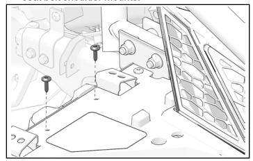
2. Install rear speaker bracket ② with retained screws. Torque two screws to specification.
