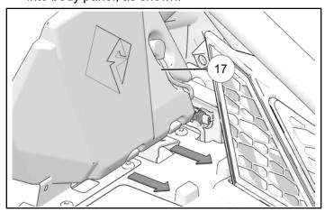
5. Install rear speaker to bracket with one knob ②).
