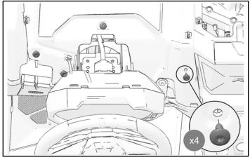
7. Install front of dashboard with three retained dashboard fasteners.
