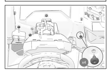
7. Install front of dashboard with three retained dashboard fasteners.
