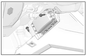
3. Install driver side panel with eight retained center console fasteners and one push-pin rivet.
