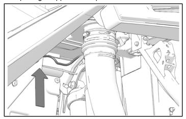
6. Install rear speaker harness towards front of vehicle with push-darts and cable ties, as needed.
