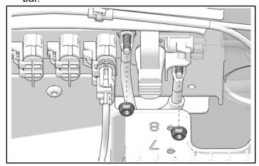
5. Install negative (black) and positive (red) onto Polaris Pulse® bar terminals with retained nuts. Torque nuts to specification.
