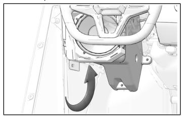
2. Install speaker with two retained screws. Torque screws to specification.
