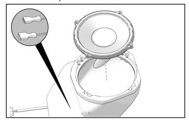
3. Connect speaker housing harness to bottom of accessory speaker (20).
