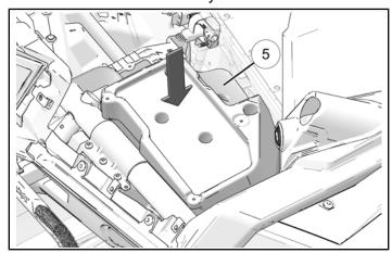
8. Install upper subwoofer housing with six screws ④ and six washers ③. Torque screws with hex key ⑥ (not shown) until screws are fully seated.
