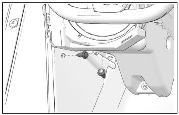
5. Remove and keep four screws attaching front dashboard to speaker.
