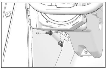
5. Remove and keep four screws attaching front dashboard to speaker.
