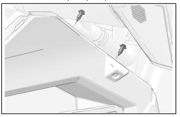
4. Carefully lift center panel upwards to remove side panels from vehicle.
