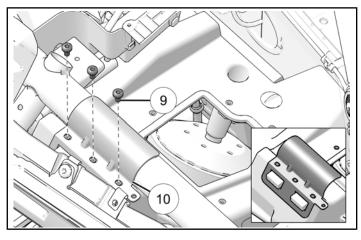
5. Install bottom of subwoofer to firewall with two screws ① and two washers ②. Torque screws to specification.
