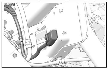
3. Route harness towards bottom opening and install edge-clip to bottom of accessory mounting tray.
