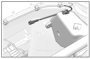
5. Remove and keep two push-pin rivets from inner side panel.
