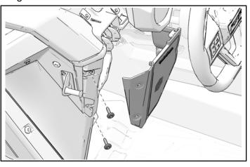
2. Remove and keep one screw attaching fender flare to front dashboard.
