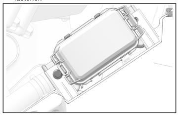
5. Rotate fuse block upwards towards front of vehicle to access push-pin rivet beneath fuse block.
