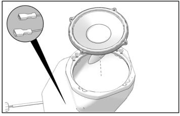
3. Connect speaker housing harness to bottom of accessory speaker @.
