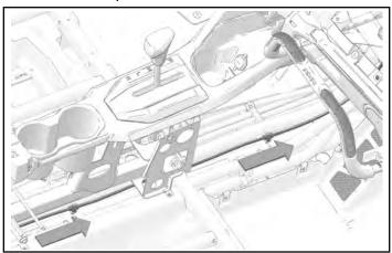
7. Install rear speaker harness to accessory mounting tray with edge-clip. Put harness around underside of mounting tray and towards rear speaker connector of the vehicle's audio harness.
