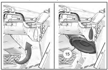
4. Put subwoofer bracket (1) onto subwoofer and over chassis tube. Install bracket to subwoofer with three screws 9.
