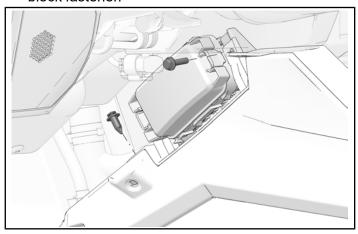
4. Loosen, but do not remove, left-hand fuse block fastener.
