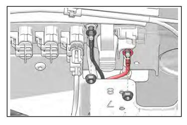
6. Route remaining harness through opening in accessory mounting tray and install connector to main audio harness.
