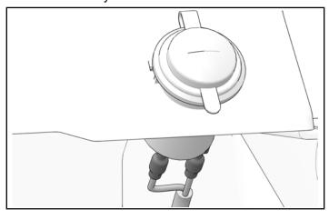
5. Remove and keep two center console fasteners from driver side.
