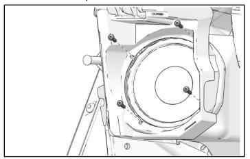
6. Remove and keep two screws attaching speaker to firewall.
