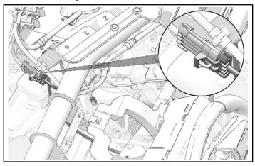
10. Two Passenger Vehicles Only: Collect excess harness with a cable tie and put in the location shown.
