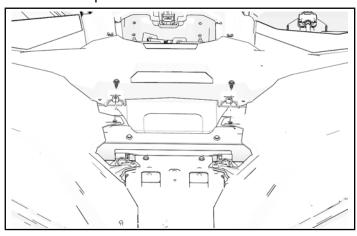
7. Carefully lift edge of left front hood panel to release tab from dashboard top as shown.
