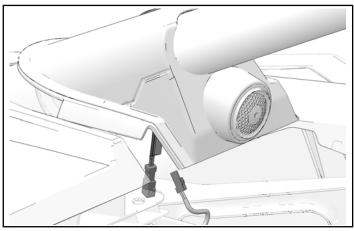
2. Slide rubber boot upwards to access tweeter.
