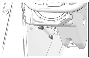
6. Install one screw attaching fender flare to front dashboard. Torque one screw to specification.
