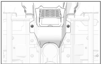
2. Remove and keep four center console side fasteners (shorter).
