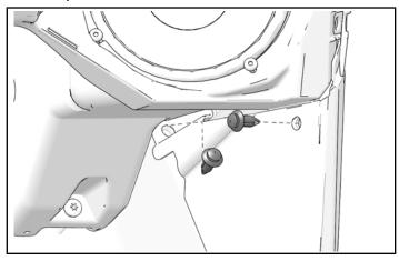
6. Remove and keep four screws attaching front dashboard to speaker.
