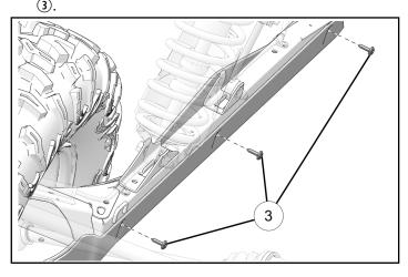
4. Torque all six trailing arm screws ③ to specification.
