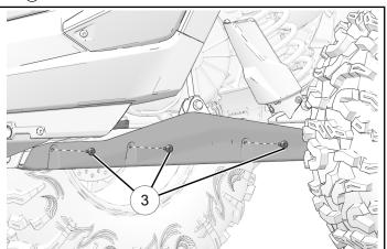
3. Loosely install inside of guard with three screws
