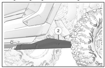
2. Loosely install outside of guard with three screws 3.
