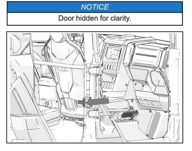
2. Remove two screws and limit strap bracket from rear of B-pillar.
