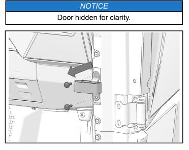
3. Close door and engage door with striker. This will help support door while hinge screws are removed.
