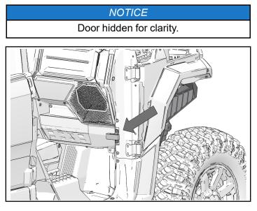
2. Remove two screws and limit strap bracket from A-pillar.
