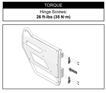
2. Install two screws (5), two nuts (6), and limit strap bracket. Tighten screws to specification.
