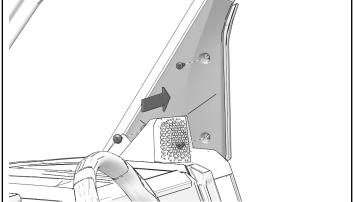
3. Install push-pin rivet.
