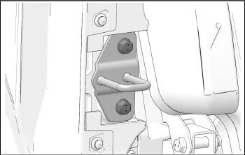
4. Put bracket through limit strap. Install bracket and two screws to B-pillar. Tighten bracket screws to specification
