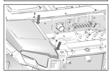
4. Install four push pin rivets.
