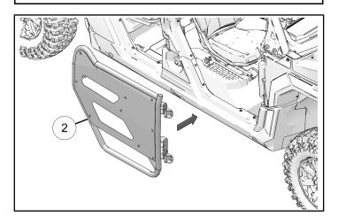
2. Loosely install four retained hinge screws.
