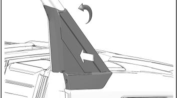
2. Install inner panel and three screws. Tighten screws to specification.
