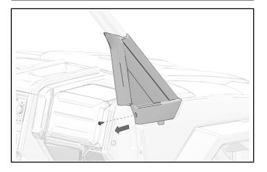
3. Remove and keep two screws from inner panel.
