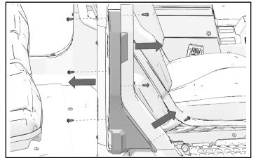
2. Turn top of trim away from vehicle. Lift trim to disengage the lower tab. Remove trim.
