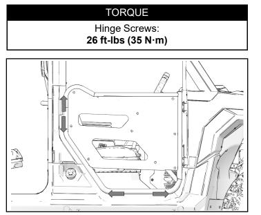
2. After door is properly positioned, check engagement with striker. Adjust striker up or down as needed for proper latching. If door rattles when latched, adjust striker up or down to slightly load door. If door is difficult to open, adjust striker outward. Remove striker cover to access striker screws.
