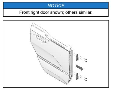
2. Remove and keep two screws and limit strap bracket from inside of door.
