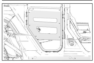
2. After door is properly positioned, check engagement with striker. Adjust striker up or down as needed for proper latching. If door rattles when latched, adjust striker up or down to slightly load door. If door is difficult to open, adjust striker outward. Remove striker cover to access striker screws.
