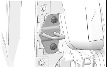
4. Put bracket through limit strap. Install bracket and two screws to A-pillar. Tighten bracket screws to specification
