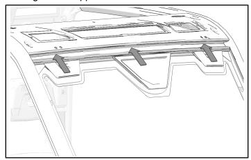
3. Engage upper windshield clamps (§) into grooves on windshield mount.
