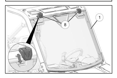
4. Adjust seal on left side and right side of windshield to cover edge of windshield and A-pillars.
