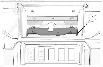
2. Install backer bracket ④ to upper chassis bar with two screws ⑤.
