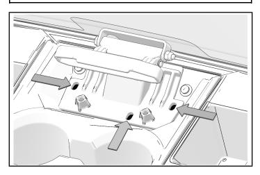
8. Install three screws **(6)** through windshield bracket and cup holder.
