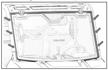
5. Loosely install two upper windshield clamps ® to upper ROPS bar with four carriage bolts ⑨ and four nuts ⑩.
