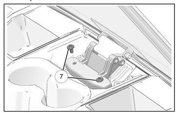
3. Torque clamp screws to specification.
