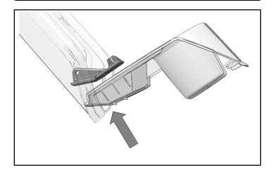
3. Use windshield bracket as a template to mark three holes on cup holder.
