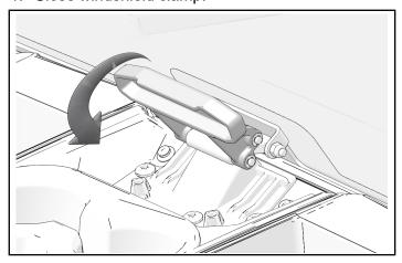
2. Install two windshield clamp screws ① through clamp and into windshield bracket.
