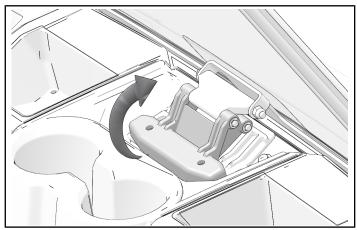
7. Align holes on windshield bracket with drilled holes in cup holder.
