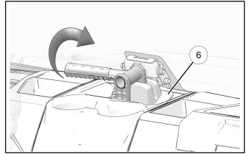
2. Move windshield handle forward and align handle legs over handle base <sup>(6)</sup> in the vented position, as shown.
