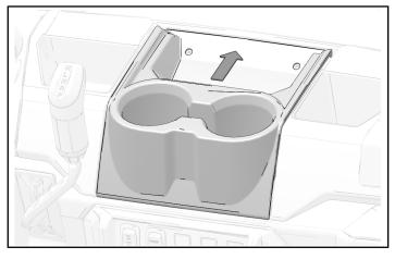
2. Install cup holder with two retained push-pin rivets.
