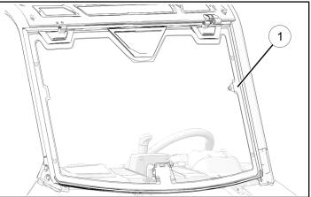
3. Move pin on left side windshield hinge into bushing on left side windshield mount <sup>(1)</sup>.
