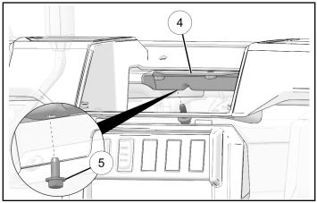
NOTICE Dash has been hidden to show backer bracket installation location on chassis bar.
