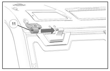
5. Install right side windshield mount (1) to upper ROPS with two screws (3) and two nuts (9).
