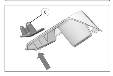
2. Use handle base (6) as a template to mark three holes on cup holder.
