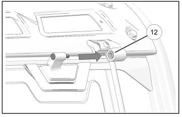
4. Install right side windshield mount bushing (1) onto right side windshield hinge pin.
