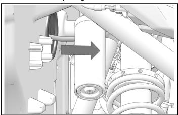
12. Install one edge clip to chassis, above suspension.
