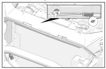
17. Put all display connectors in between brackets. Install one push-dart to chassis tube.
