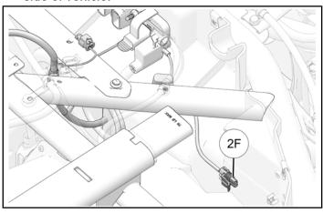
6. Remove and keep one nut from negative terminal on Polaris Pulse® bar.
