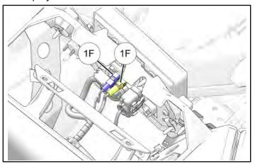
11. Install the AM/FM antenna connector into the back of the Ride Command® display.
