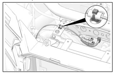
14. Install one push-dart to chassis tube, located behind headlight and beside radiator shroud.
