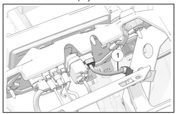
13. Attach edge clip ② to the dashboard support bracket, as shown.
