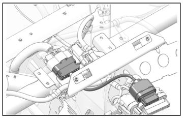
20. Install infotainment connector **16M** to main vehicle harness.
