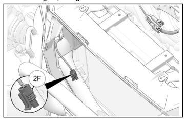
16. Route front camera connector under top of radiator shroud. Install one push-dart to radiator shroud.
