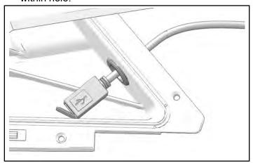
5. Install storage compartment with four retained fasteners. Torque fasteners until fully seated.
