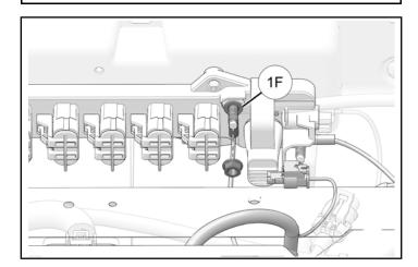
8. Remove and keep one nut from positive terminal on Polaris Pulse® bar.
