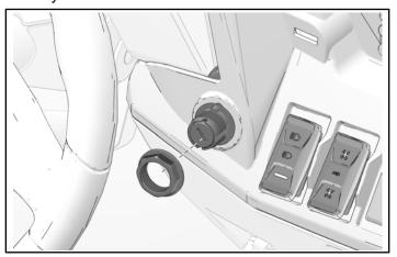
6. Install bezel with two retained lower bezel fasteners.
