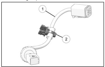
4. Put USB harness through hole in storage compartment and make sure grommet is seated within hole.
