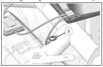
4. Install antenna connector to Ride Command® harness.
