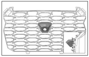
2. Install camera mount on grille, as shown.
