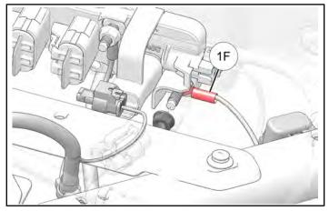
10. Put ambient air temperature sensor connector, front camera connector, and GPS antenna connectors through firewall grommet.
