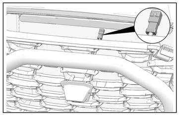
6. Put bottom of grille in first and push top of grille in until two tabs engage upper front fascia.
