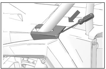
2. Slide flat head screwdriver under front pocket fender.
