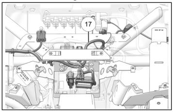
2. Attach push-dart to diagonal chassis tube.
