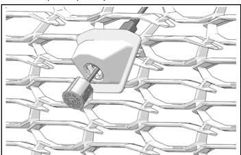
4. Find front camera connector on underside of radiator shroud. Remove cap from connector.
