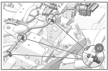
23. Rear audio equipped vehicles only: Remove cap from rear audio connector on main vehicle harness.
