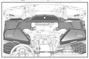
2. Install upper dashboard with five fasteners.
