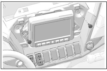
7. Install bezel with two retained upper fasteners.
