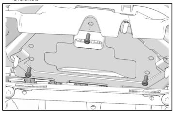
2. Remove four fasteners holding gauge bracket to bezel.
