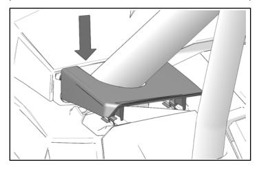
4. Gently push tab into clips until front pocket fender is secure.
