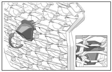
3. Put front camera into mount and push until two side clips snap into place.
