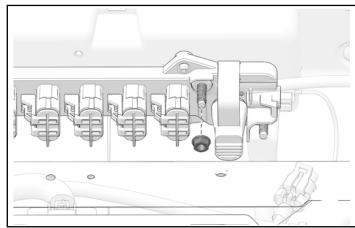
7. Install negative ring terminal **1F** (black) to Polaris Pulse® bar with retained nut. Torque nut to specification.
