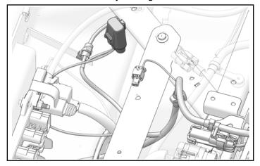
4. Install one edge clip to ridge on firewall.
