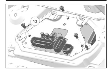
3. Put bezel near dashboard. Reach behind bezel and connect all switches and 12 V connections.
