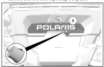
2. Find rear camera connector on chassis electrical harness and remove cap.
