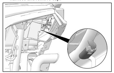
3. Connect rear camera to chassis electrical harness.
