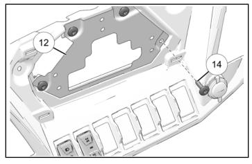
2. Install Ride Command® display (sold separately) to display bracket with three fasteners ③. Torque three fasteners to specification.
