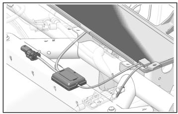
3. Install ground ring to chassis tube with screw 3.
