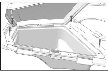
2. Drill one **1 in (25 mm)** hole for the USB grommet in the driver side dashboard storage compartment along witness line.
