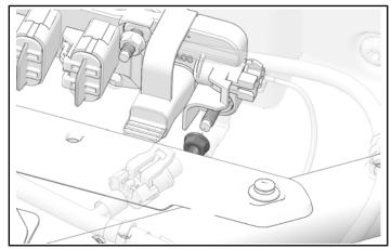
9. Install positive ring terminal **1F** (red) to Polaris Pulse<sup>®</sup> bar with retained nut. Torque nut to specification.
