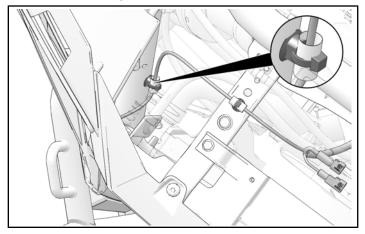
15. Route ambient air temperature sensor connector **2F** through opening in radiator shroud.
