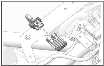
24. Rear audio equipped vehicles only: Install rear audio connector **4M** to main vehicle harness.
