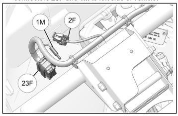
22. Install harness to chassis with three edge clips.
