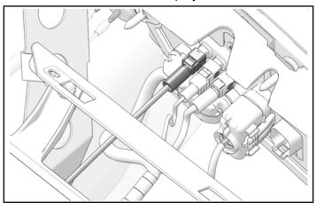
12. Install the USB harness ① into the back of the Ride Command® display.
