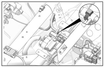
18. Install subwoofer connector **4F** to chassis tube.
