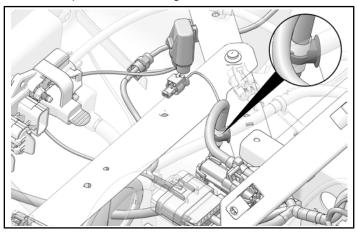
3. Attach fuse assembly to diagonal tube.
