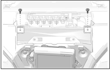
8. Torque four bezel fasteners to specification.
