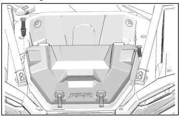
3. Lock & Ride® assemblies may need adjustment. Tighten or loosen bottom nut depending on fitment.
