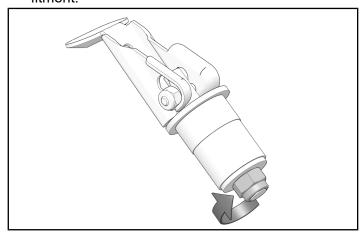
4. Make sure Lock & Ride® assemblies are fully seated before closing top lever and securing storage box.
