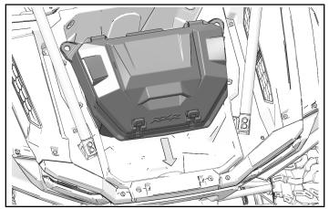
2. Install two Lock & Ride® assemblies in two aligned mounting holes.
