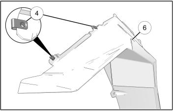
2. Align fender flare <sup>(6)</sup> with vehicle and loosely install to chassis tube with three screws <sup>(3)</sup>.
