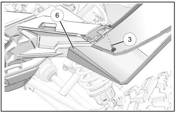
5. Torque all front fender flare screws ③ and ④ to specification.
