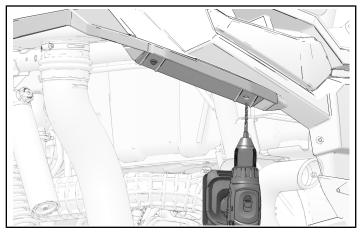
7. Install left rear fender flare (5) to rear fascia with one push-pin darts (8).
