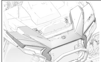
2. Install outer hood fasteners with four retained fasteners. Torque the four fasteners to specification.
