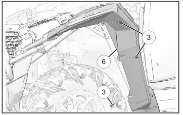
Loosely install front fender flare 6 with two screws
