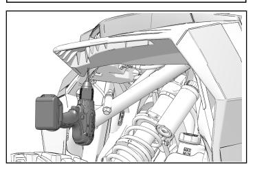
Align fender flap the with lower fender flare and install with four push-pin darts (8).
