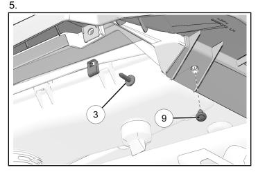
Push rear of fender flare 5 inward and align with rear fascia.
