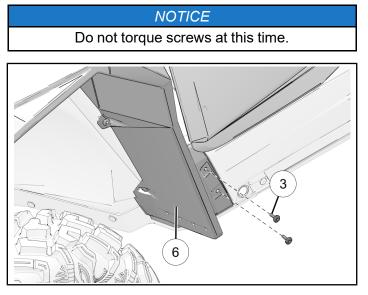
Make sure top mounting point of fender flare 6 is behind upper front fascia and install with one screw 3.
