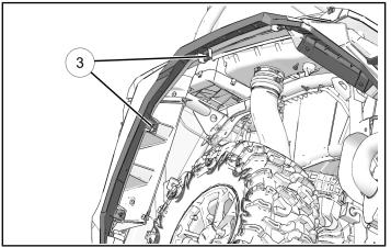
4. Install screw (9) followed by screw (3). Torque to specifications.
