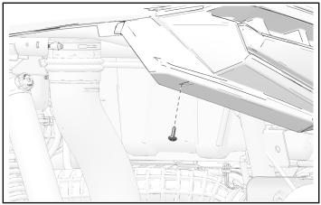
2. Install five U-nuts ④ onto rear fender flare ⑤
