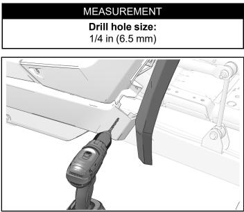
11. Install lower fender flare with two screws (9). Torque two screws to specification.
