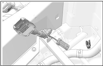
6. Counter-hold nut and remove one bolt to remove buckle assembly from vehicle. Discard hardware and seat belt buckle.
