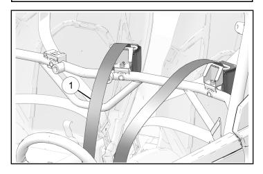
3. Put alignment tab in harness guide and put shoulder straps in guides, as shown.
