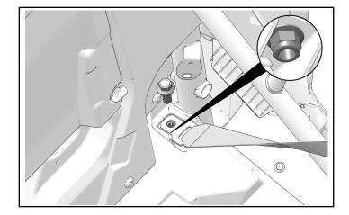
3. Remove and discard one bolt, one washer, and one nut holding harness guide.
