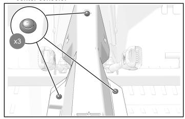
6. Remove three fasteners from the right-side of the center console.
