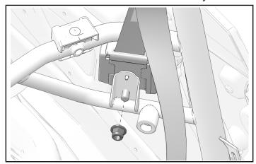
2. Counter-hold nut and remove one bolt from lower mounting position.
