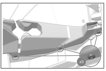
3. Install rear of center console with three retained push-pin rivets.
