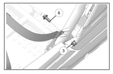
6. Install inside mounting position with one bolt 6 and one nut 3. Counter-hold nut and torque bolt to specification.
