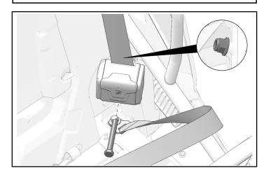
2. Counter-hold nut and remove one bolt holding lower mounting bracket. Discard hardware.
