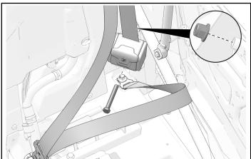
2. Counter-hold nut and remove one bolt holding lower mounting bracket. Discard hardware.
