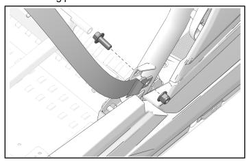
3. Remove and discard one bolt, one washer, and one nut holding harness guide.
