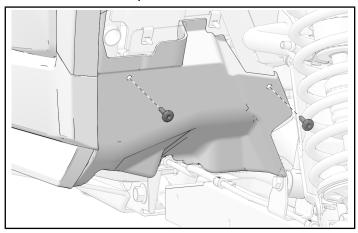
3. Remove wheel well shield from vehicle.
