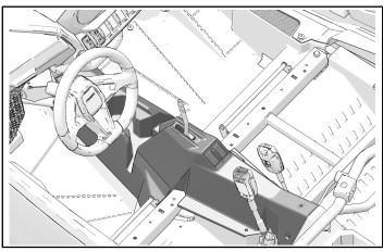
2. Install passenger side of center console with three retained fasteners.
