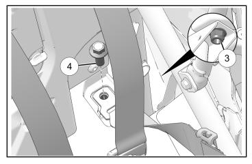
4. Install inside mounting position with one bolt ④ and one nut ③. Counter-hold nut and torque bolt to specification.
