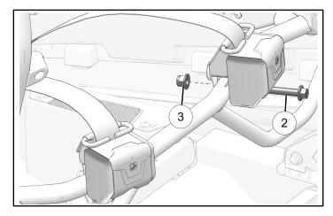
5. Install outside mounting position with one bolt ⑥ and one nut ③. Counter-hold nut and torque bolt to specification.
