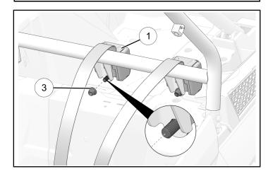
3. Install outside mounting position with one bolt 4 and one nut 3. Counter-hold nut and torque bolt to specification.
