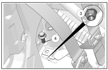
4. Install inside mounting position with one bolt 4 and one nut 3. Counter-hold nut and torque bolt to specification.
