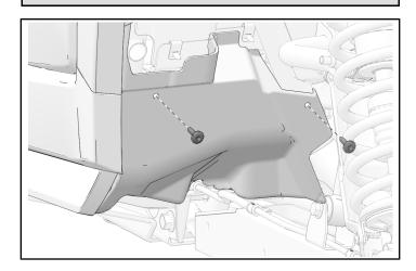
3. Install bottom of shield with two retained push-pin rivets
