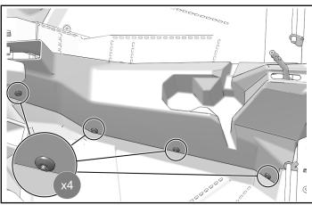
5. Remove three push-pin rivets from the rear of the center console.
