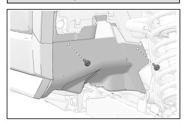
3. Install bottom of shield with two retained push-pin rivets.
