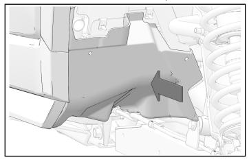
2. Install top of shield with two retained screws.
