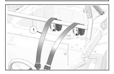
2. Install retractors with two bolts ② and two nuts ③. Counter-hold nuts and torque two bolts to specification.
