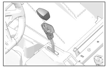
2. Remove and keep one fastener from shifter handle.
