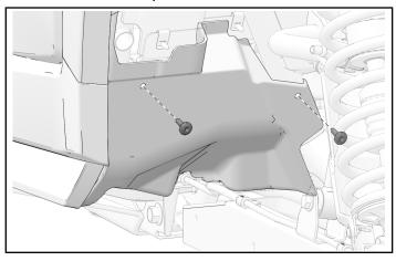
3. Remove wheel well shield from vehicle.
