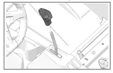
7. Install shifter handle with one retained fastener. Torque fastener to specification
