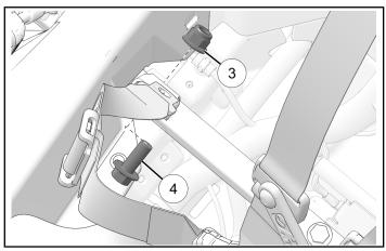
5. Driver Side Only: Connect seat belt switch harness to main vehicle harness.
