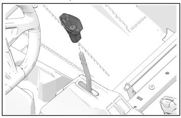
4. Remove four fasteners from the left-side of the center console.
