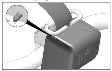
4. Install retractors with two bolts ② and two nuts ③. Counter-hold nuts and torque two bolts to specification.
