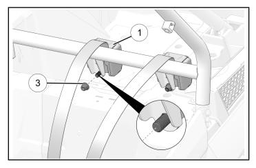
3. Install outside mounting position with one bolt ④ and one nut ③. Counter-hold nut and torque bolt to specification.
