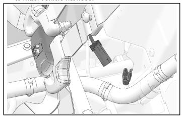
6. Install front mounting positions with two bolts ⑤. Torque bolts to specification.
