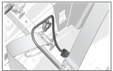
8. Install front mounting positions with two bolts ①. Torque bolts to specification.
