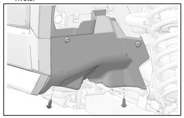
4. Torque two screws to specification.
