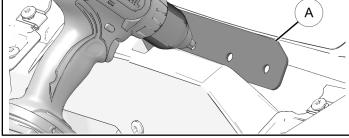
3. Attach bracket (A) using five push pin rivets (B).
