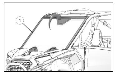
5. Attach glass windshield at top of ROPS using two screws ④ and two nuts ⑤. Torque to specification.
