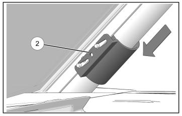
7. Attach windshield clamp ② with screw ⑧. Torque to specification.
