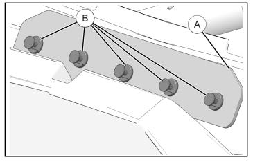
4. Install glass windshield assembly ① onto bracket
