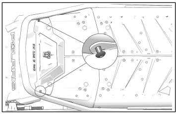
2. Pull out slightly on sides of bumper and remove from the machine.
