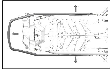
3. Install the new bumper. Pull out on the sides of the bumper slightly to help installation.
