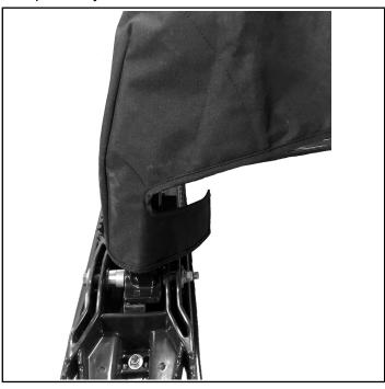
4. Connect the straps under the lower suspension arms.
