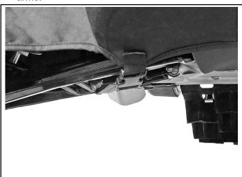
5. Connect the right rear strap to the left corner of the rear bumper. Then connect the left rear strap to the right corner of the rear bumper. The straps will cross under the tunnel.
