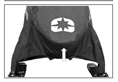
3. Put hook and loop fastener around the suspension spindles, just above the ski.
