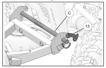
3. Once plow frame is fully seated onto the mounting bar make sure the locking plates are rotated into position to allow the locking pins (4) to be inserted.
