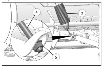
• In the event of a collision with an obstacle at a speed greater than that recommended for the system, the shear pin ① of the manual angle mechanism ® will break to minimize the force of impact in the frame. If the shear pin is broken, inspect the plow system for damaged parts. If any part is damaged, the impact velocity was greater than what the system is designed to support. You must then buy a replacement part from your dealer.
