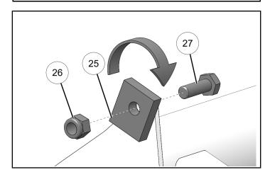
2. Make sure both blade adjuster blocks are mounted in the same position. Tighten until fully seated.
