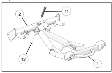
2. Insert the clevis pin ① of the plow pivot from top down through the center pivot and secure by placing the cotter pin ② through the hole at the bottom of the pin.
