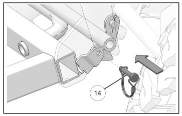
4. Insert the locking pins and latch the lanyard (15) and lanyard choke (16) to secure the pins in place.
