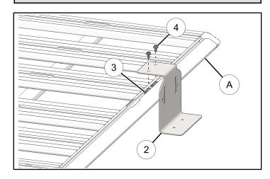
4. Attach pioneer u-bracket ① to pioneer side bracket ② with two screws ④.
