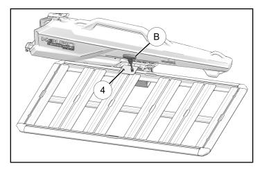
4. Adjust angle of gun boot to desired position.
