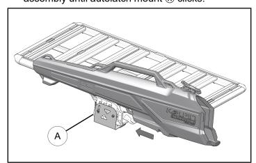
2. Slide assembly to desired position.
