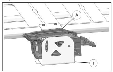
3. Loosely install autolatch mount (A) to pioneer ubracket (1) with two screws (5) and two nuts (6).
