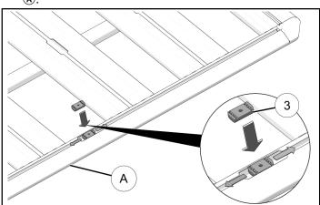
2. Slide both channel nuts 3 to desired location.
