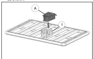
2. Align holes on autolatch mount (A) with holes on pioneer u-bracket (1).
