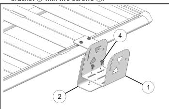
5. Torque two pioneer side bracket screws ④ with torque tool ⑧ or torque to specification using socket set.
