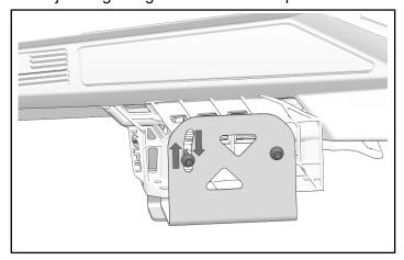
5. Counter hold nuts and torque two screws ⑤ to specification.
