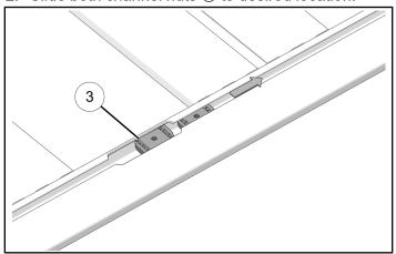
3. Loosely install pioneer side bracket ② to platform rack frame ⓐ with two screws ④ and the two channel nuts ③.
