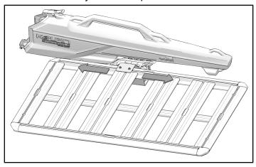
3. Torque two pioneer side bracket screws ④ with torque tool ⑧ or torque to specification using socket set.
