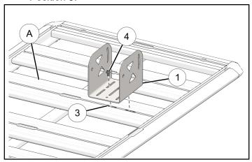
4. Torque two screws ④ with torque tool ⑧ or torque to specification using socket set.
