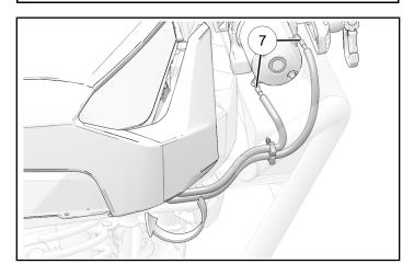
14. Pull cables ① up through hole near radiator cap and attach to yellow winch contactor to yellow terminal and blue winch contactor to blue terminal. Secure with provided nuts and torque to specification.
