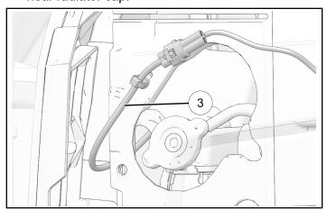
10. Connect winch jumper harness ③ to main vehicle harness near radiator.
