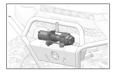
2. Install four screws ① and torque to specification.
