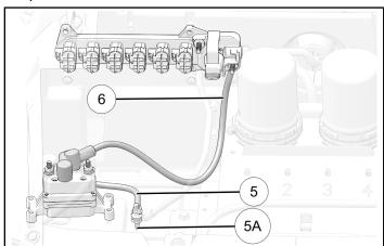
20. Secure both cables with provided nuts and torque to specification.
