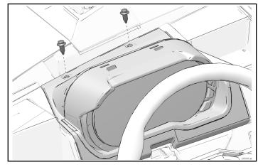
2. Remove the instrument cluster by pulling straight out towards the steering wheel.
