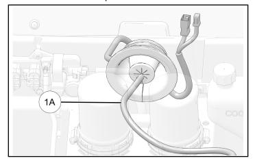
23. Locate pre-wired main harness connector under dash. Remove harness tape if necessary to access connector and connect to receiver harness.
