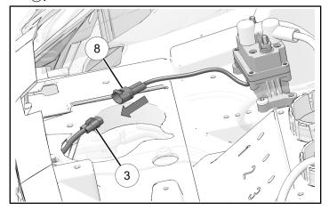
9. Route winch jumper harness ③ down through hole near radiator cap.
