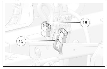
24. Connect switch harness ② to receiver harness and route under dash to open accessory switch on drivers side of dash.
