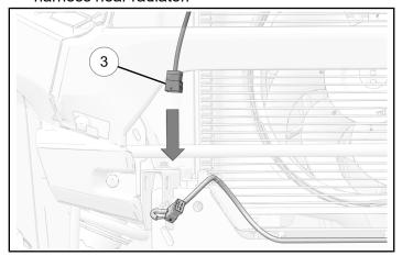
11. Remove cable clip from winch cable ①.
