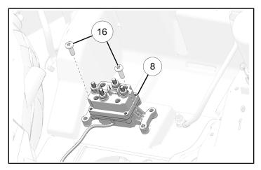
8. Route contactor harness ® to the front of the vehicle and connect to the winch jumper harness ③.
