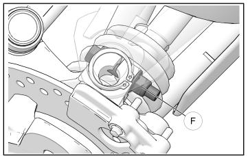
6. Pull the lower A-Arm downward so that the upper A-Arm <sup>(G)</sup> disconnects from the knuckle assembly.
