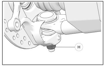
8. Rotate/flex the knuckle assembly rearward to allow the lower A-Arm ball joint ① to be lifted from the knuckle assembly.
