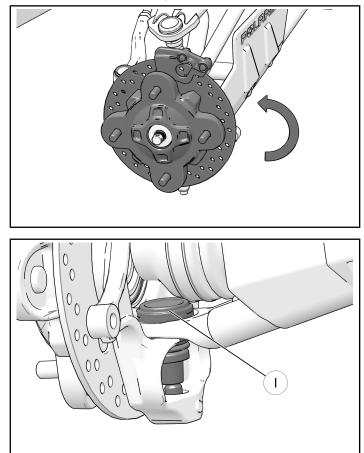
9. Remove the nut ①, washer, and bolt from the rear bracket holding the lower front A-Arm.
