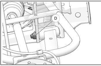
5. Repeat this procedure for the opposite side of the vehicle to remove the other lower rear A-Arm.
