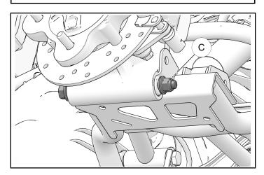
4. Attach the suspension to the A-Arm using the retained nut (1) and bolt. Torque to specification.
