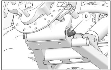
3. Remove the nut <sup>(C)</sup>, washer, and bolt holding the lower rear A-Arm to the front bracket.
