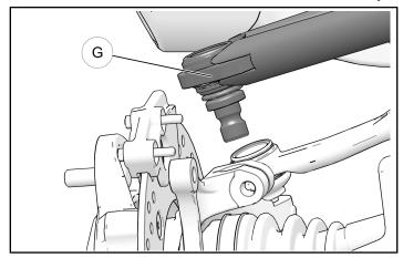
7. Remove the nut (#) holding the lower A-Arm ball joint in place.
