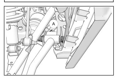
Install into the rear bracket using the retained nut
