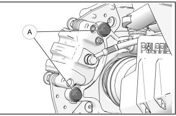
2. Remove the brake caliper (B) and hang it on the vehicle frame using a bungee cord, wire, or similar item to prevent stress on the brake line (C).
