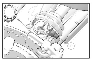
8. Install the brake caliper using the two retained bolts (H). Torque to specification.
