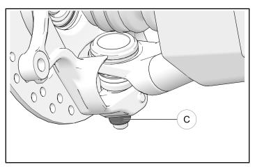
4. Install castle nut (1) on the axle. Torque to specification.
