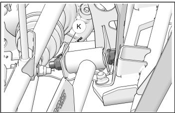
11. Repeat this procedure for the opposite side of the vehicle to remove the other lower front A-Arm.
