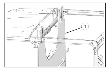
3. Loosely install storage panel strap around left side and right side of rear grab bar (A) and attach with buckles.
