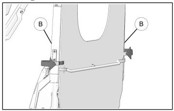
5. Install three lower storage panel straps around lower chassis bar © behind the bottom of the front seats and attach with buckles.
