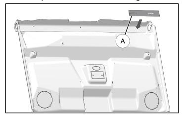
3. Set template (A) to the far right of the roof ROPS trough.
