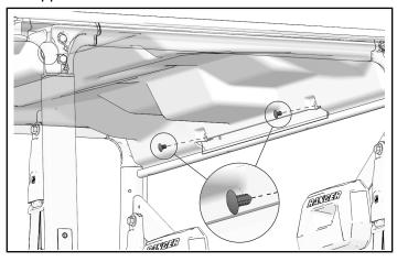
5. Remove and keep two screws and two washers from center of rear roof liner.
