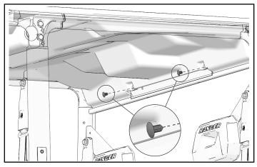
11. Install four retained screws into center of rear roof liner.
