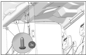
3. Remove and keep four screws from center of rear roof liner.
