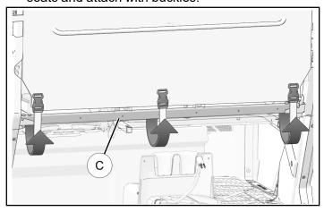
6. Tighten all straps for a snug fit on vehicle.
