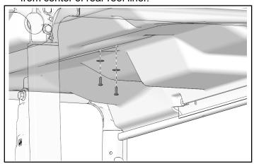
Carefully pull left-hand and right-hand edges of rear roof liner down from between ROPS and roof seal.
