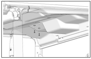
10. Install two retained push darts through liner and upper rears ROPS bar.
