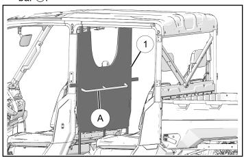
2. Attach two upper left side and two upper right side hook-and-loop straps on storage panel ① around upper ROPS bar.
