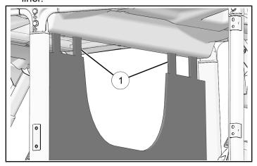
8. Attach two upper left side and two upper right side hook-and-loop straps on storage panel ① around upper ROPS bar.
