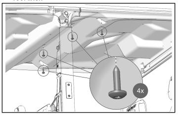
4. Remove and keep two push darts from liner and upper rear ROPS bar.
