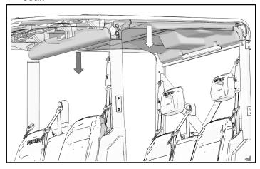
7. Remove rear edge of roof liner from the roof support channel.
