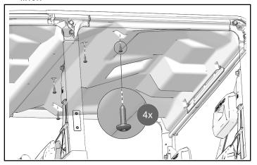
12. Install three retained screws through liner below center ROPS bar.
