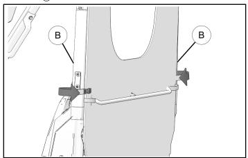
4. Install three lower storage panel straps around lower chassis bar © behind the bottom of the front seats and attach with buckles.
