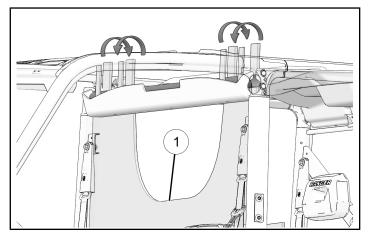
9. Install two retained screws and two retained washers into center of rear roof liner.
