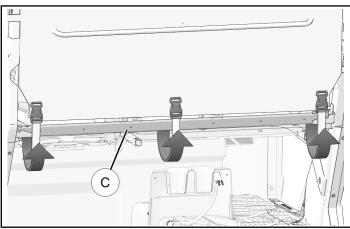
5. Install rear edge of roof liner into roof support channel.
