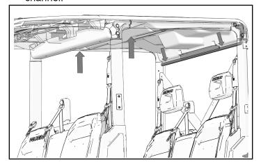
6. Carefully push left-hand and right-hand edges of rear roof liner up between ROPS and roof seal.
