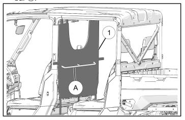
2. Loosely install storage panel strap around left side and right side of rear grab bar (A) and attach with buckles.
