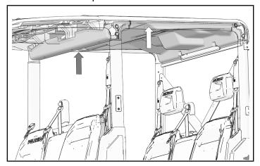
7. Put two upper left side and two upper right side hook-and-loop straps ① through cut-outs in roof liner.
