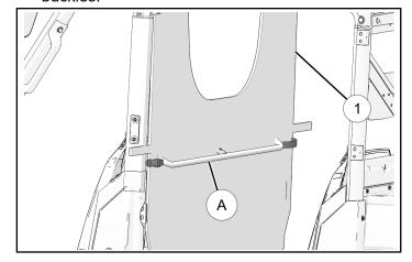
4. Loosely install left side and right side storage panel straps around left side and right side B-pillar bars (B) and attach with buckles.
