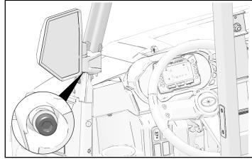
2. Install mirror plate ③ with two screws ④.
