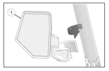
3. Tighten screws until fully seated.
