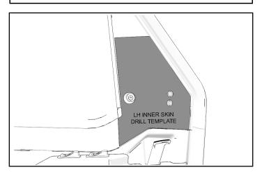
3. Align bolt cut-out on template over the bolt on the inside of door.
