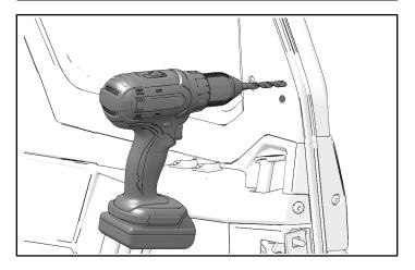
8. Drill larger spacer hole through each pilot hole on outside of door.
