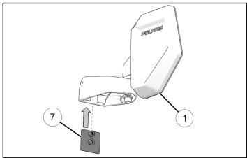
2. Install the mirror assembly 1 to the door with two screws (5).
