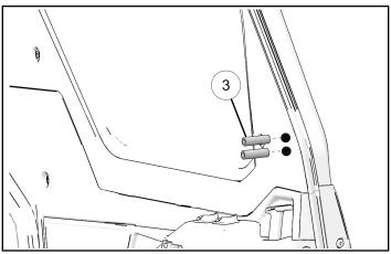
2. Install mirror backer plate ④ to the inside of the door with two screws ⑥ through two spacers ③.
