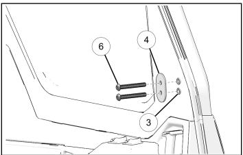
3. Slide weld nut backer plate  $\mathcal{D}$  into mirror arm  $\mathbb{O}$ .
