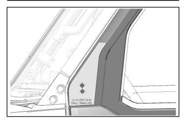
2. Tape inner skin template to inside edge of driver side door, as shown.
