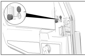
2. Drill one hole through each pre-marked indentation on the inside of the door.
