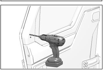
7. Drill pilot hole through the center of each marked location on the inside of door.
