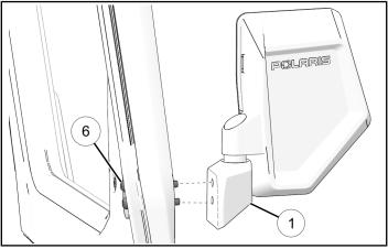
5. Torque screws to specification.
