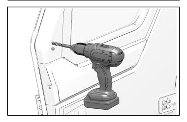
9. Drill larger spacer hole through each pilot hole on inside of door.
