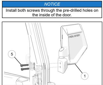
3. Torque screws to specification.
