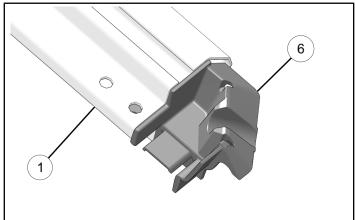
6. Slide two side extrusions ② into each corner base.
