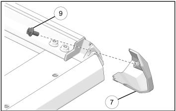
10. Torque all bolts with torque tool 10.
