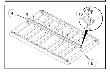
2. Torque all bolts sequentially from one end with torque tool ①.
