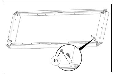
8. Loosely install four platform planks  $\ \ \,$  in to platform frame assembly with sixteen bolts  $\ \ \,$   $\ \ \,$
