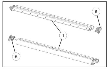
5. Insert left-hand corner base pieces ⑥ inside the channel on each end of extrusion ①.
