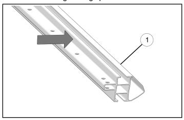
2. Install two right-hand corner base pieces ⑤ to front and rear extrusions ⑴.
