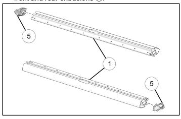
3. Insert right-hand corner base pieces ⑤ inside the channel on each end of extrusion ①.
