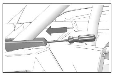
3. Gently lift screwdriver upward to free front pocket fender from clips.
