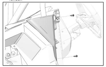
2. Turn rear pocket fender away from vehicle body and remove.
