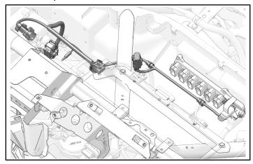
2. Install fuse relay into driver-side diagonal tube.
