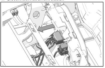
2. Remove and keep ignition switch retaining nut.
