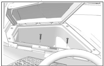
6. Install two storage compartment fasteners. Torque fasteners until fully seated.
