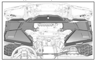
2. Install upper dashboard with five fasteners.
