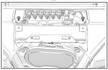
7. Torque four bezel fasteners to specification.
