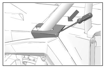
2. Slide flat head screwdriver under front pocket fender.
