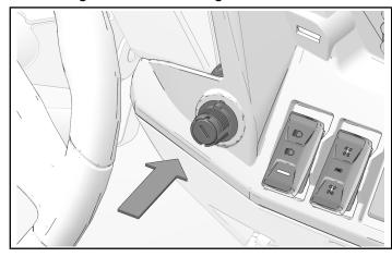
4. Disconnect 12V port on right-hand side, if installed.
