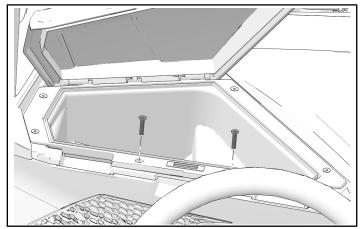
5. Remove and keep five fasteners from front of upper dashboard.
