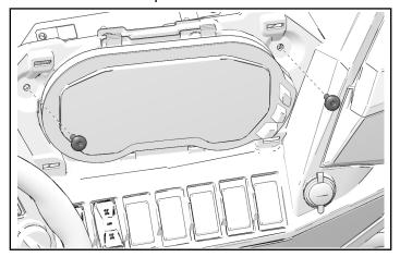
7. Carefully pull bezel away from dashboard. Reach behind bezel and disconnect all remaining electrical connections.
