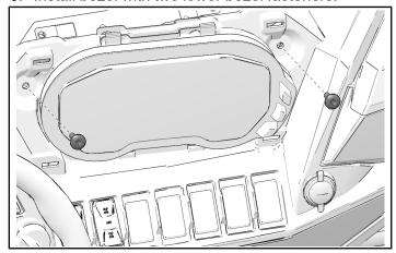
6. Install bezel with two upper fasteners.
