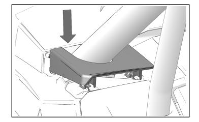
4. Gently push tab into clips until front pocket fender is secure.
