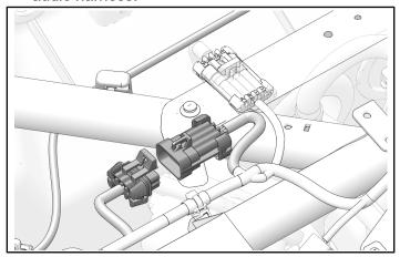
9. Install amplifier level connector **8F** to PMX audio harness.
