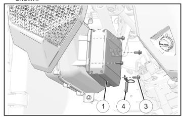
2. Install amp connector 23F and ground connector 1M to amplifier.
