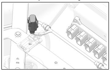
3. Install harness to ridges on firewall with two edge clips.
