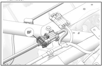
10. Remove and keep cap from amplifier connector on PMX audio harness.
