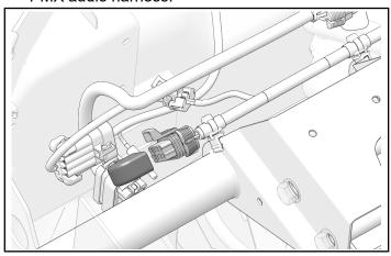
11. Install amplifier connector **7M** to PMX audio harness.
