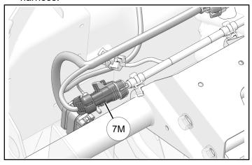
12. Install retained cap on output connector on PMX harness.
