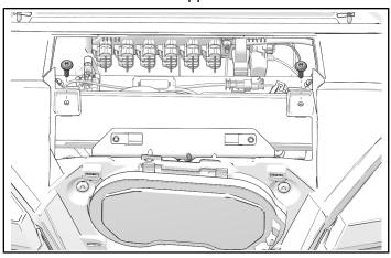
7. Torque four bezel fasteners to specification.
