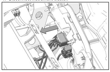
2. Remove and keep ignition switch retaining nut.
