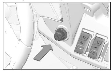
4. Disconnect 12V port on right-hand side, if installed.
