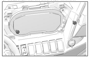
6. Install bezel with two upper fasteners.
