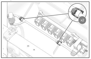
4. Remove and keep one nut from negative terminal on Polaris Pulse® bar.
