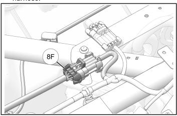
10. Remove and keep cap from amplifier connector on PMX audio harness.
