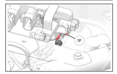
8. Disconnect amplifier level connectors on PMX audio harness.
