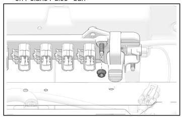
5. Install negative ring terminal **1F** (black) to Polaris Pulse® bar with retained nut. Torque nut to specification.
