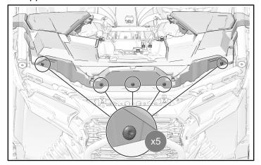
6. Remove and keep two fasteners from top of upper dashboard.
