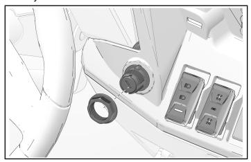
5. Install bezel with two lower bezel fasteners.
