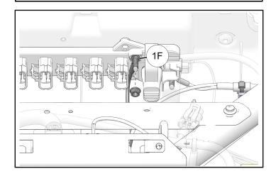
6. Remove and keep one nut from positive terminal on Polaris Pulse® bar.
