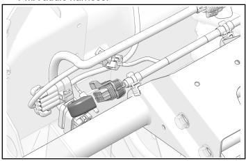
11. Install amplifier connector **7M** to PMX audio harness.
