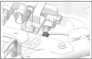
7. Install positive ring terminal **1F** (red) to Polaris Pulse<sup>®</sup> bar with retained nut. Torque nut to specification.
