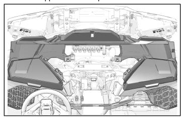
2. Install upper dashboard with five fasteners.
