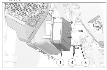
2. Install amp connector **23F** and ground connector **1M** to amplifier.
