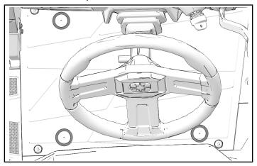
2. Install six spacers ③ with screws ④ in dimpled locations.
