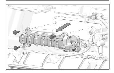
6. Put AM/FM antenna bracket (6) in between chassis plate and pulse bar plate.
