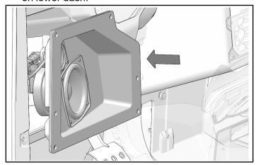
9. Install left side speaker grille ⑤ to right side speaker assembly and to lower dash compartment with six screws ①.
