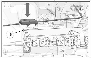
10. Attach antenna harness to chassis bar with one screw (7).
