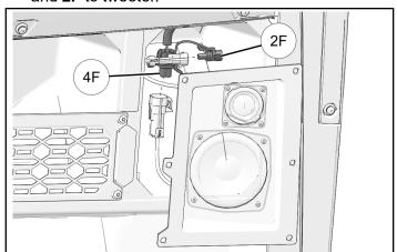
9. Carefully place speaker assembly into speaker compartment on lower dash.
