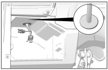
5. Install speaker harness edge clip to the chassis bar located inside of upper dash.
