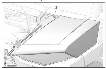
2. Remove and keep one push-pin rivet from outer hood.
