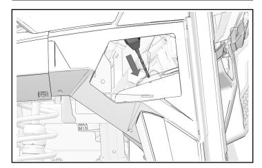
3. Route speaker harness ③ through hole in speaker compartment on lower dash.
