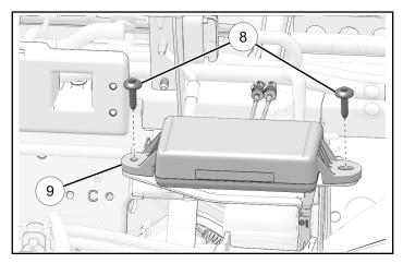
2. Connect V2V and GPS connections to harness.
