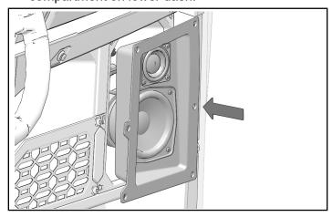
10. Install right side speaker grille ② to right side speaker assembly and to lower dash compartment with six screws ①.
