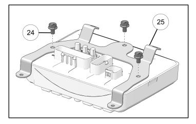
2. Install bracket (25) with display onto display bezel (26) with two screws (1). Torque to specification.
