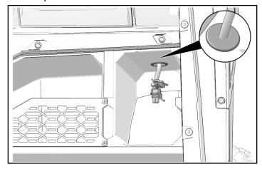
6. Install speaker harness edge clip to the chassis bar located inside of upper dash.
