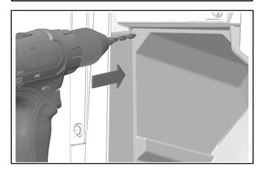
2. Drill speaker harness hole through dimple on outside of speaker compartment on lower dash.
