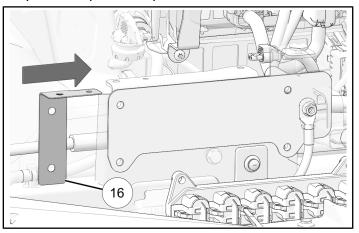
7. Install AM/FM antenna bracket (6) and pulse bar to chassis bar with two bolts (8) and one retained pulse bar bolt.
