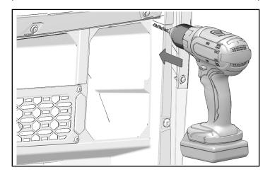
2. Drill pilot hole through the dimple on the outside of the speaker compartment on lower dash.
