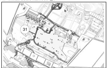
2. Install harness cable ties to electric mount panel locations, as shown.
