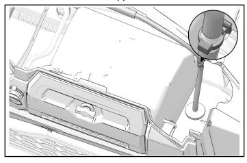
7. Install speaker seal ④ onto backside of speaker ③.
