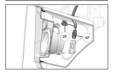
8. Set speaker assembly into speaker compartment on lower dash.
