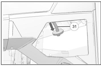
4. Install grommet into harness hole in speaker compartment on lower dash.
