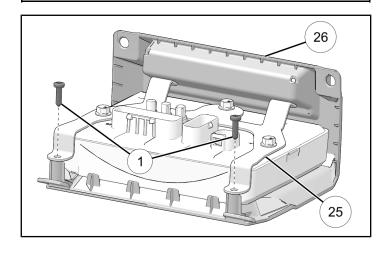
3. Install two push-pin rivets ② through bracket with display and through display bezel.
