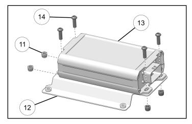
2. Install amplifier bracket ② to the backside of the electrical mount with four screws ⑩. Torque to specification.
