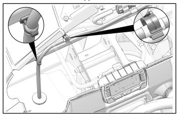
6. Install speaker seal ① onto backside of speaker6.
