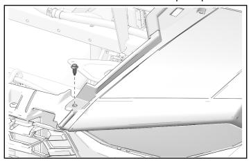
3. Attach rear of outer hood with one retained screw. Torque outer hood screws to specification.
