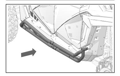
5. Torque four fasteners (8) to specification.
