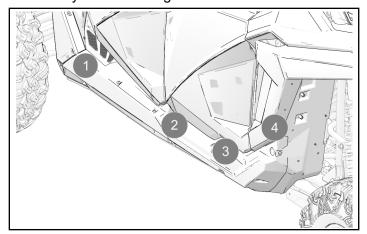
4. Put anchor assemblies into chassis mounting locations.
