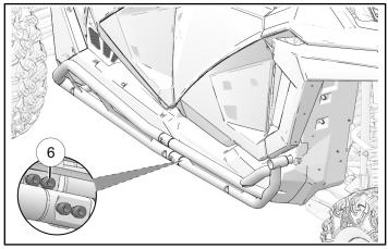
8. Install three small diameter plugs ① and one large diameter plug ⑤ into rock slider.
