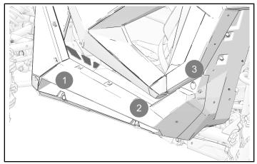
3. Put anchor assemblies into chassis mounting locations.
