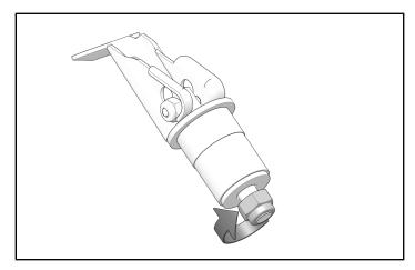
5. Close each Lock & Ride® anchor latch to install cooler mount.
