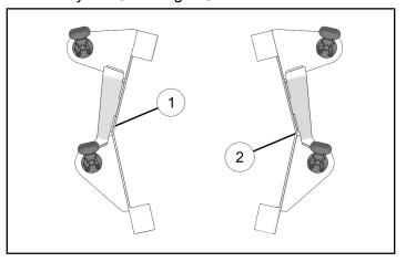
3. Put cooler (sold separately) in cargo box and open lid. Align cooler mount bracket with cargo box and cooler, as shown.
