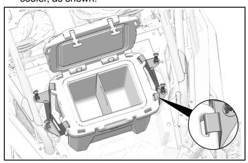
4. Lock & Ride® assemblies may need adjustment. Tighten or loosen bottom nut depending on fitment.
