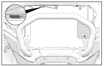
5. Put grille against bumper and install front camera to electrical harness.
