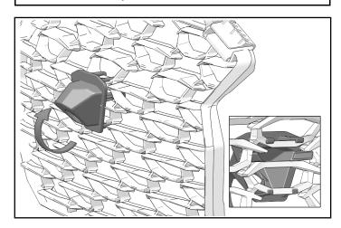
3. Put front camera into mount and push until two side clips snap into place.
