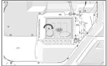
4. Slide front seat rearward to engage rear mounts. Lower front of seat.
