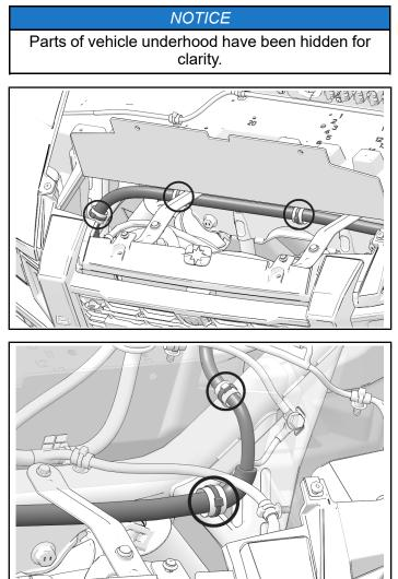
4. Locate outer grommet in upper tray and put end of harness with power cable and multiple connectors through grommet.
