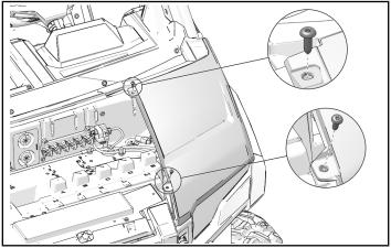
4. Install two push pin rivets in top of front fender.
