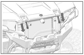
3. Put grill mounting tabs in openings on front fascia. Install top of grill on hood.
