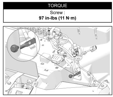
11. Locate the four-pin connector on the chassis harness near the pulse bar and remove the blank plug from the connector.
