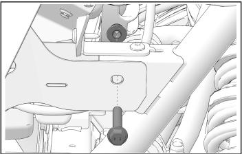
6. Loosely install two screws in the lower mounting holes.
