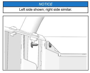
3. Remove rear plate of HD bumper by pulling outward.
