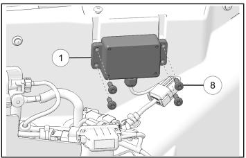
2. Attach autostop box 1 to winch control harness 2 as shown.
