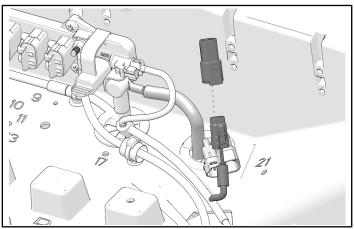
12. Connect chassis harness connector to matching winch harness connector.
