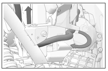
3. Loosely install winch assembly ③ to accessory bumper using four kept screws ⑩.
