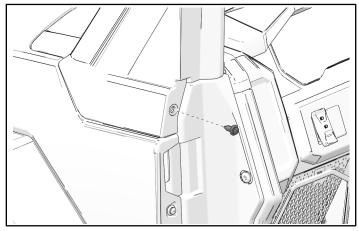
4. Remove outer sail panel by turning and pulling outward.
