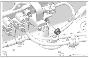
7. Install terminal ring end of positive cable (red) to Pulse<sup>®</sup> bar stud. Attach with kept nut and torque nut to specification.
