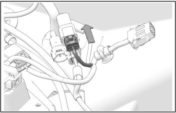
14. Connect 4F connector into the mating connector of the main winch harness.
