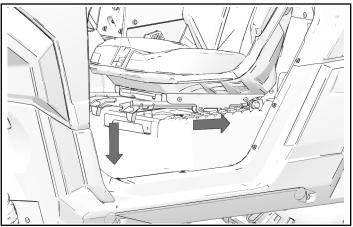
5. Install two screws at front of seat base. Torque screws to specification.
