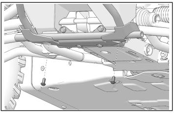
8. Torque middle mounting screws to specification.
