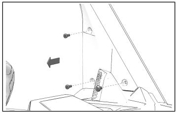
3. Remove push pin rivet from outer sail panel.
