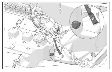
10. Install negative terminal end (black wire) so center hole lines up and it is 90° off from the already present terminal. Attach with kept screw and torque to specification.
