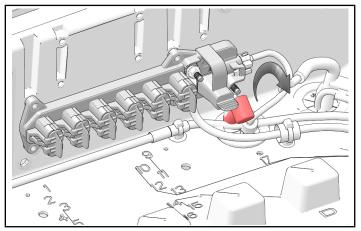
6. Remove and keep nut from positive Pulse® bar terminal ring.
