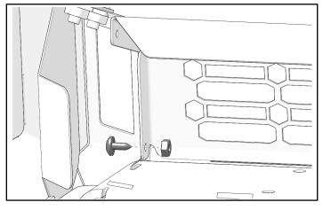
5. Remove top plate of HD front bumper by lifting up and pulling outward.
