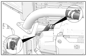
2. Route harness across top of core support as shown. Install cable clip ties into core support as shown.
