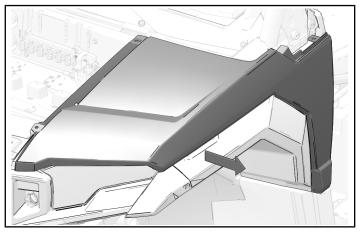
6. Turn fender and lift to disengage lower tab and remove fender.
