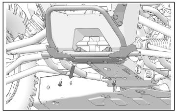
3. Remove and keep two screws from lower mounting holes.
