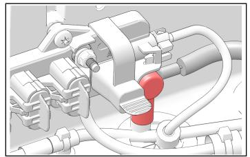
9. Remove and keep screw (9) from negative terminal end body connection.
