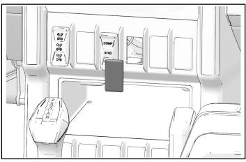
2. Locate empty connector for winch control switch and pull connector through blank opening. Empty connector will have a winch icon.
