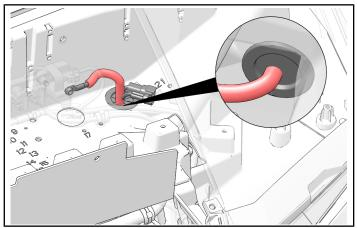
5. Remove boot from positive connector and move boot out of way to access nut.
