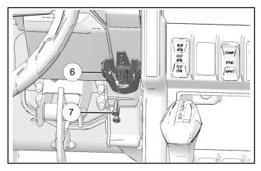
2. Put remote control ④ into remote control holder ⑥.
