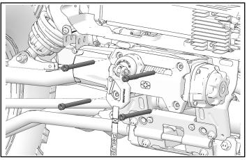
Disconnect all harness connections and remove 4500 Pro HD winch by lifting upward and pulling outward.
