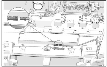
2. Remove two push-pin rivets from the front of the underhood liner.
