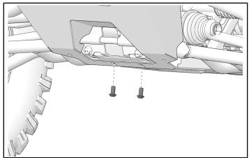
7. If machine is equipped with snowplow mounting plate, loosely install two additional screws in the lower mounting holes.
