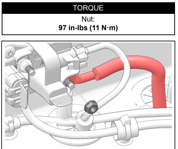
8. Install rubber boot onto positive terminal post.
