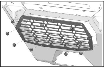
2. Remove and keep two screws and two nuts from the top of the top plate of the HD front bumper.
