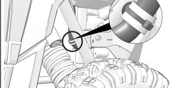
3. Continue to route harness along top of core support. Install cable clip ties into core support as shown.
