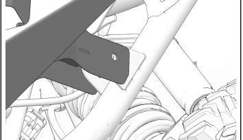
4. Loosely install four screws and four nuts to secure the middle mounting points.
