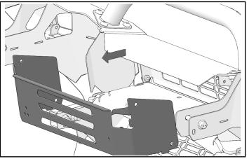
4. Remove and keep two screws and two nuts from the bottom of the HD front bumper.
