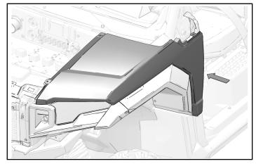
3. Install two screws in front fender. Tighten until fully seated
