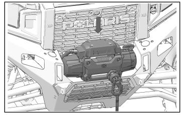
2. Route the harness through the HD front bumper and above the frame as shown.
