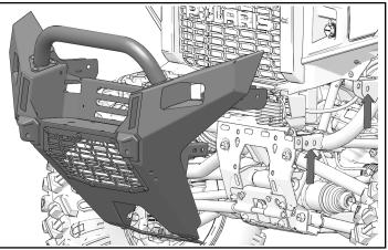
2. Middle mounting point slides into the bracket in the vehicle frame.
