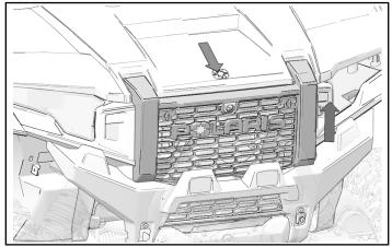
3. Unhook the rubber straps for the hood. Lift the hood to remove.
