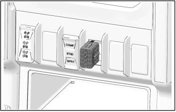
Install new winch control switch (5) to open connector and install into blank opening in dash. Push into opening until a click is heard.
