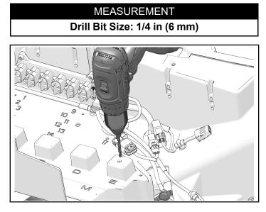
16. Clip fuse block into "E" mounting point into previously drilled hole.
