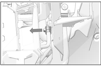
2. If machine is equipped with snowplow mounting plate, remove and keep two screws from lower mounting holes.
