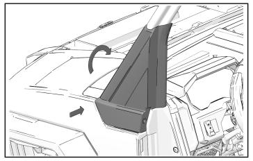
2. Attach inner sail panel using three screws and torque screws to specification.
