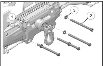
6. Torque screws to specification in the order shown below.
