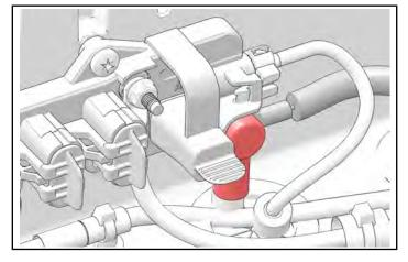
9. Remove and keep screw from negative terminal end body connection.
