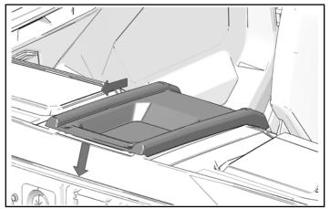
2. Install two push-pin rivets.
