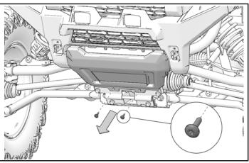
2. Pull bottom of winch cover down to disengage the top tabs. Remove winch cover.
