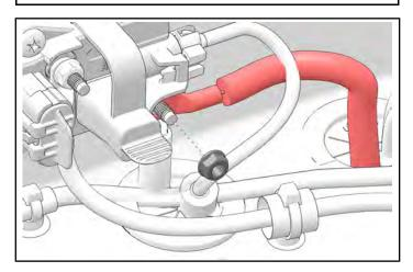
8. Install rubber boot onto positive terminal post.
