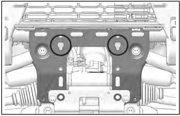
3. Install winch assembly ① onto notched holes and pull wire harness through as winch is moved into place.
