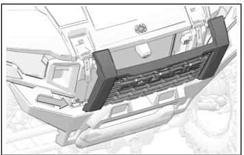
4. Push each stud in and turn one-quarter turn clockwise to secure the grill.
