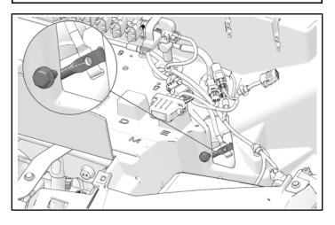
11. Locate the four-pin connector on the chassis harness near the pulse bar and remove the blank plug from the connector.
