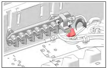
6. Remove and keep nut from positive Pulse<sup>®</sup> bar terminal ring.
