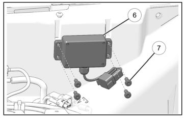
2. Attach autostop box connector (6) to winch control harness (8) as shown and clip harness to vehicle frame using fir tree clip.
