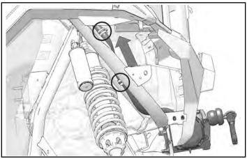
2. Route harness across top of core support as shown. Install cable tie clips into core support as shown.
