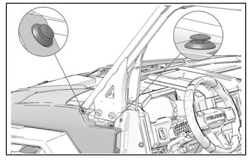
5. Install two push pin rivets in rear edge of front fender.
