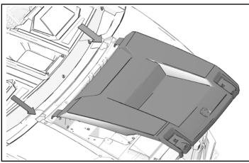
2. Pull the rubber straps down over the hooks to secure the hood.
