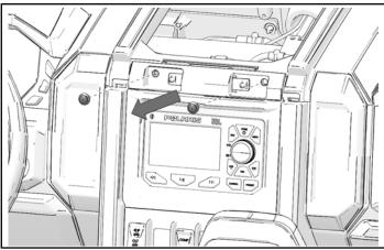
2. Rotate top of head unit away from dash and lift head unit to remove from dash.
