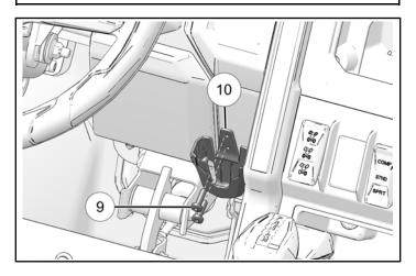
2. Put remote control (1) into remote control holder (10).
