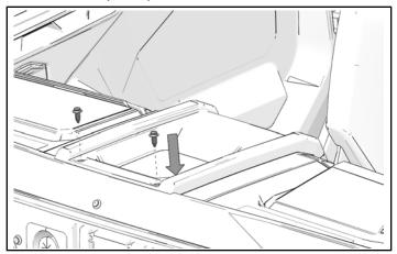
3. If vehicle is equipped with tip-out windshield. Install base, three screws, and washers. Tighten screws to specification.
