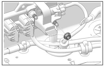
Install terminal ring end of positive cable (red) to Pulse<sup>®</sup> bar stud. Attach with retained nut and torque nut to specification.
