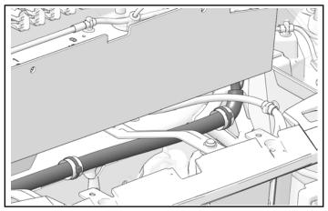
4. Locate outer rubber grommet in upper tray and insert end of harness with power cable and multiple connectors through grommet.
