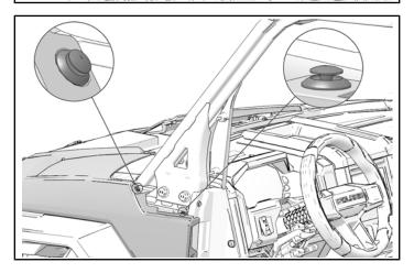
3. Remove and keep two push pin rivets from top of front fender.
