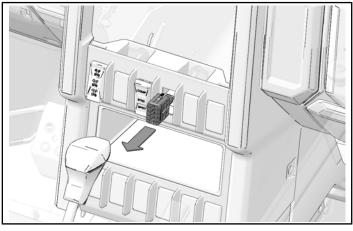
Install new winch control switch ④ to open connector and install into blank opening in dash. Push into opening until a click is heard.
