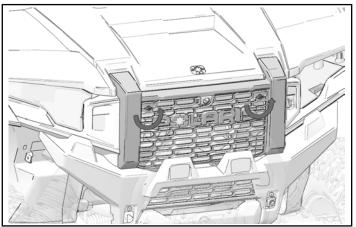
2. Pull the top of the grill forward and then lift up to remove the grill.
