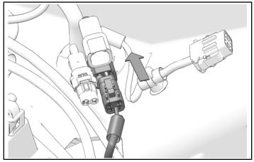
13. Connect auxiliary harness connector to matching winch harness connector.
