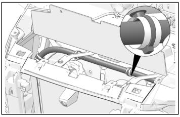
3. Continue to route harness along top of core support. Install cable ties as shown.
