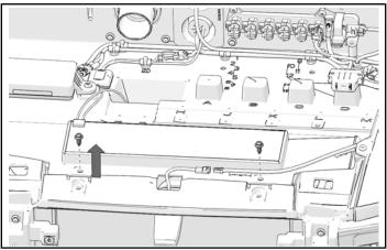
3. Lift the front panel of the underhood liner to access the areas beneath.
