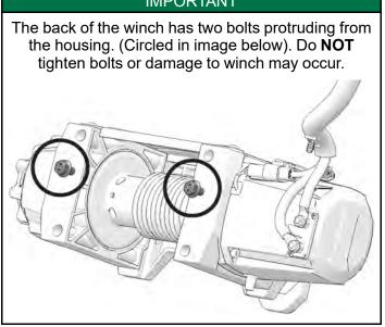
1. Set the winch assembly in front of the vehicle and route the winch harness through the bumper and over the frame.
