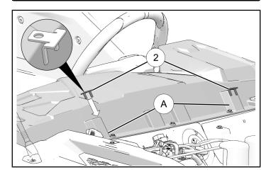
2. Use mount ② as a template to mark holes on each upper dash tab ④.
