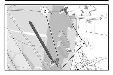
4. Drill hole through topside of each upper dash tab.
