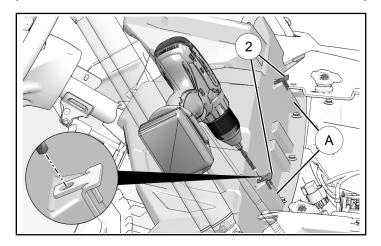
5. Install two windshield support mounts ② to upper dash tabs ④ using two push pin rivets ③.
