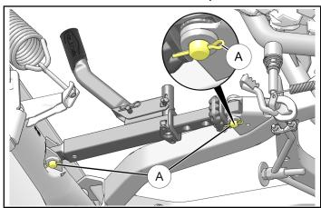
2. Remove and discard two clevis pins <sup>®</sup> from each end of manual angle adjustment mechanism.
