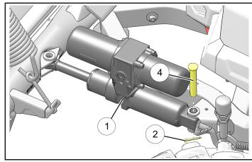
5. Attach connector on angle cylinder ① to mating TILT connector from Plow Controller.
