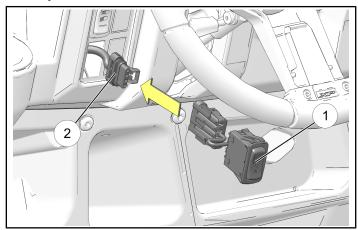
3. The other end of the jumper cable connects to the main harness at the center of the console. Route the jumper cable through the pre-made holes (A) along the interior.
