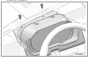
2. Tilt the instrument cluster towards the steering wheel and disconnect the instrument cluster from the chassis electrical harness.
