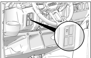
2. Pull the winch jumper cable ② through the rectangular cutout from inside the dash and connect to the winch switch ①. Once connected, push the switch into the rectangular cutout until fully seated with an audible click.
