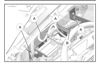
4. Attach the jumper cable ② to the winch connection © at the center of the console.
