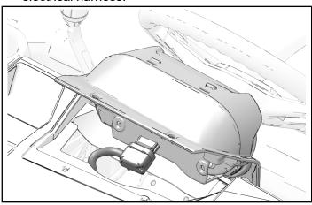
2. Install the instrument cluster bezel with two retained push-pin rivets.
