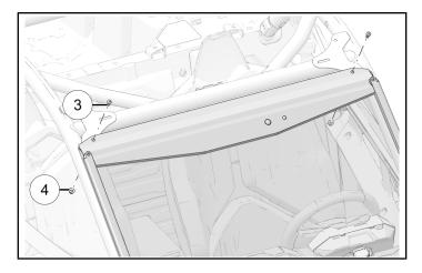
Aluminum roof-equipped vehicles: Install top of windshield with retained roof hardware. Torque fasteners to specification.
