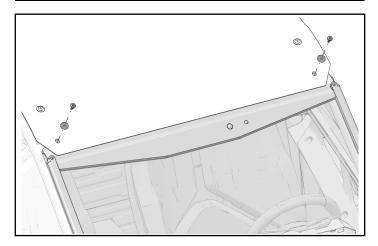
3. Install clamps ⑤ around roll-cage and install with one sleeve ⑥ and one fastener ⑦ per clamp. Torque fasteners to specification.
