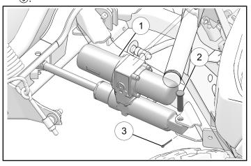
5. Attach connector on angle cylinder to mating **TILT** connector from Plow Controller.
