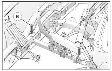
3. Remove and discard manual angle adjustment mechanism from plow frame brackets.
