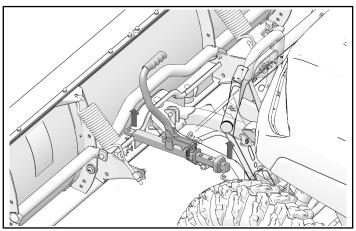
Install rearward end of angle cylinder ① to plow frame brackets using clevis pin ② and cotter pin ③.
