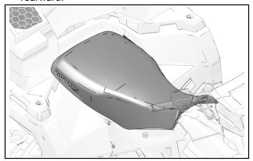
2. Identify center of hole location on rear cab as shown. Drill a 1 in hole in that location.
