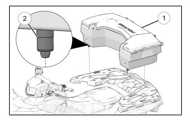
5. Attach rear storage box by rotating Lock & Ride anchor handles down into the locked (horizontal) position as shown.
