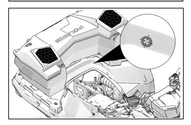
3. Insert wire harness connector through hole and install grommet **1.6** into hole.
