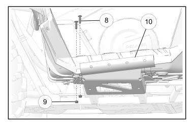
4. Slide the rear left-hand side guard weld ⑦ into the left-hand bracket mount ⑩ and lift the assembly into place.
