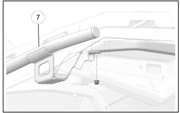
6. Loosely install the two rear footwell tube screws ④ and nuts 1 to hold the assembly into place.
