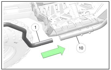
9. Loosely install the front footwell tube screws ④ and nuts <sup>①</sup>.
