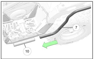
Align the bracket on the rear left-hand side guard weld ⑦ with the rear rack tube support. Loosely install the nut that was previously removed in step 1 to hold the bracket and the rear rack tube support into place.
