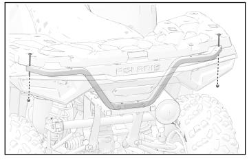
2. Remove and discard the four screws and nuts from the left footwell.
