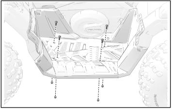
Install the left-hand bracket mount (10) onto the left footwell. Loosely install the two front footwell screws (8) and nuts (9) to hold the assembly into place.
