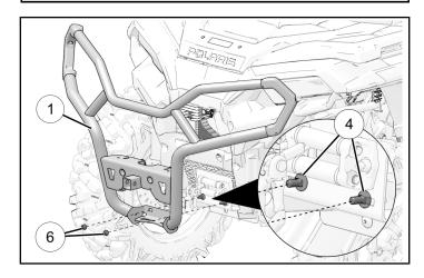
3. Install the two fasteners ③ from the front side of the front bumper into the front bumper support bracket and install the nuts ⑥ on the backside.
