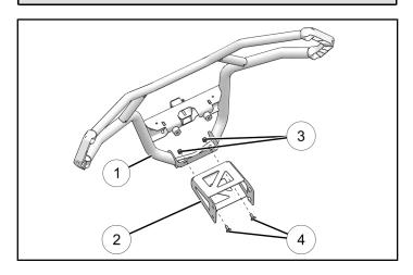
2. Install the front bumper ① / front bumper mounting bracket ② as an assembly and align mounting holes.
