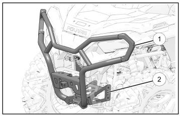
3. Install the two fasteners ③ from the front side of the front bumper into the front bumper support bracket and install the nuts ⑥ on the backside.
