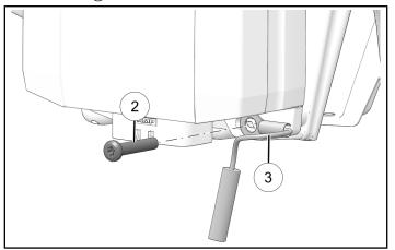
3. Torque amplifier fasteners ② to specification.
