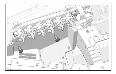
2. Install five push-pin rivets.
