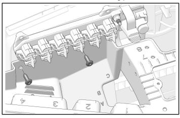
3. Move accessory mounting panel from beneath Polaris Pulse® bar and remove from vehicle.
