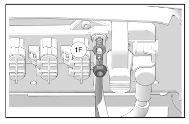
3. Install **1F** positive terminal ring (RED) to positive post. Reinstall nut and torque to specification.
