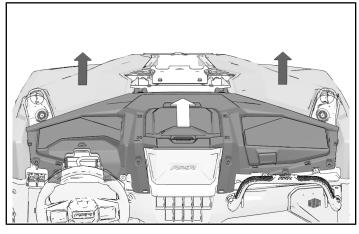
2. Ensure that tabs on panels are aligned in slots on dashboard top. (Passenger-side panel shown; driver-side panel similar.)
