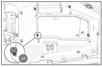
8. Install front of dashboard with three retained dashboard fasteners.
