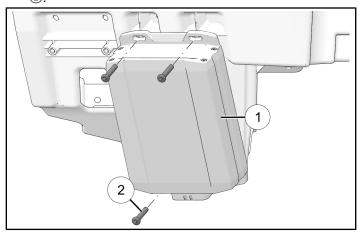
2. Install fourth fastener ② through ground jumper harness ③.
