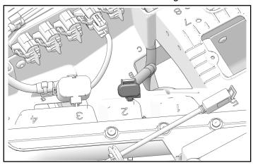
2. Disconnect amplifier output connector from speaker connector.
