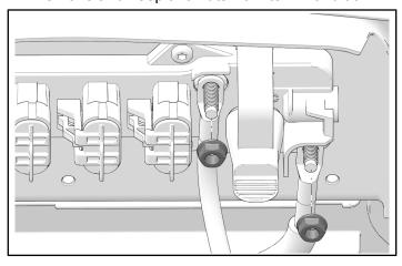
2. Install **1F** ground terminal ring (BLACK) to ground post. Reinstall nut and torque to specification.
